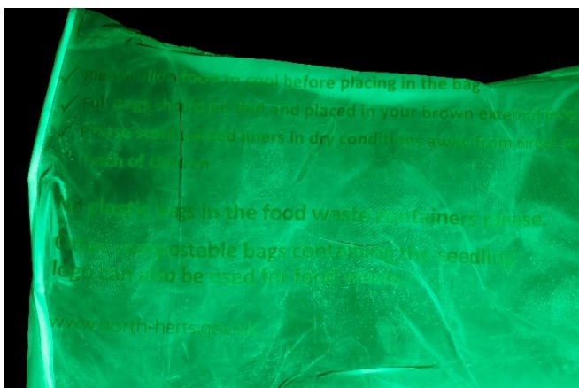
Green food disposal bag treated with Superglue Fuming then BY40 (EtOH)
