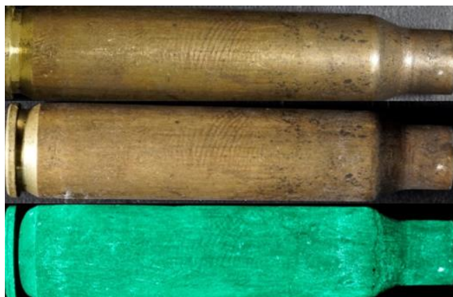
Casing imaged pre-treatment (top), after Superglue Fuming (middle) and after BY40 (bottom).
