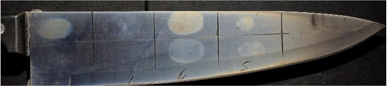
Image of Knife displaying the 'blasting' effect starting at the tip of blade.
