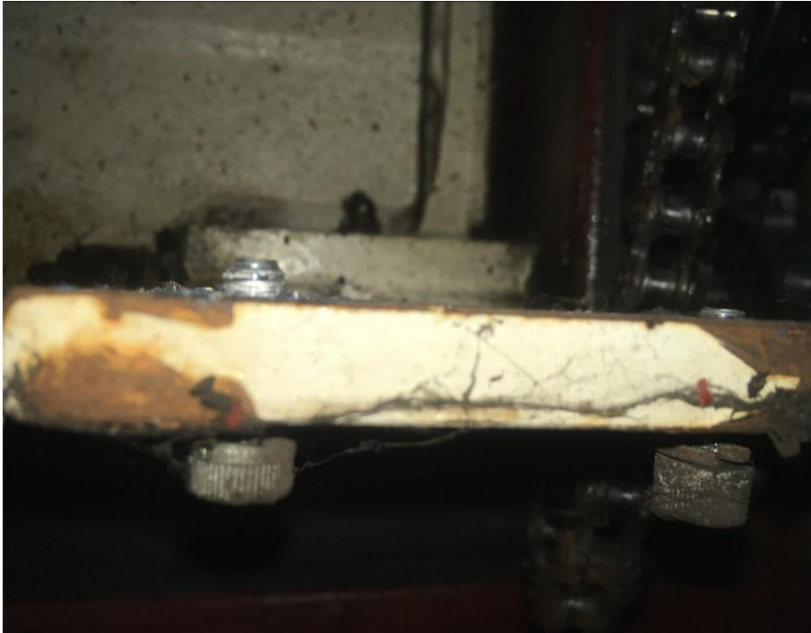
Photo 2 Showing depth of thread available to engage with door base plate
