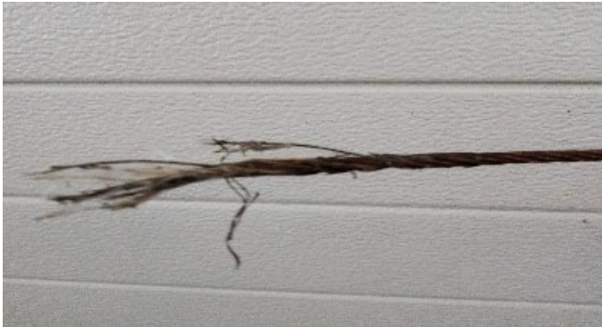
Failed galvanised cable
