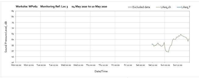
Note: Missing data from the beginning of the month until 11:00 on Saturday 9<sup>th</sup> May were due to failure of the solar panel powering the monitor.
