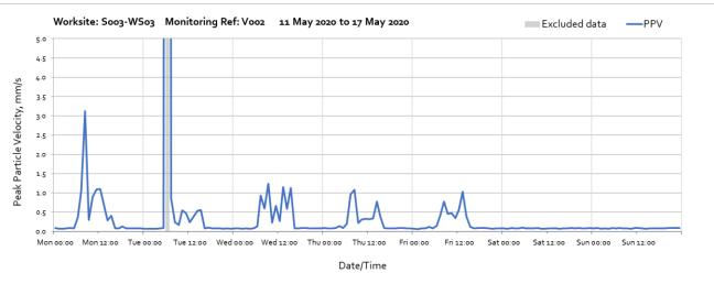
Note: High vibration levels measured at 06:00 on Tuesday 12<sup>th</sup> May were due to local disturbance of the vibration monitor and are not representative of HS2 vibration levels.
