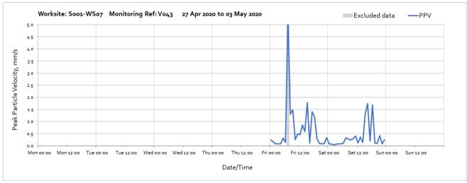
Note: High vibration levels measured at 07:00 on Friday 1st May were due to local disturbance of the vibration monitor and are not representative of HS2 vibration levels. Missing data from Sunday 3<sup>rd</sup> May until the end of the momenth was due to depletion of the monitoring station battery; access to the monitor for battery replacement was not available due to site restrictions related to Covid-19.
