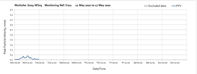
Note: Missing data from Tuesday 12<sup>th</sup> May until the end of the month were due to depletion of the monitoring station battery; access to the monitor for battery replacement was not available due to site restrictions related to Covid-19.
