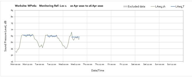
Note: Missing data between 17:00 on Thursday 22<sup>nd</sup> April and end of month were due to failure of the solar panel powering the monitor.
