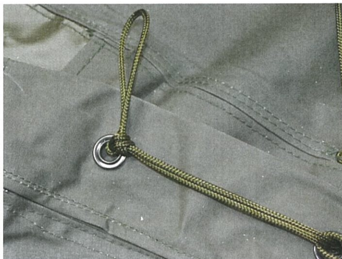
Fig 11 Dutch lacing, step 7
