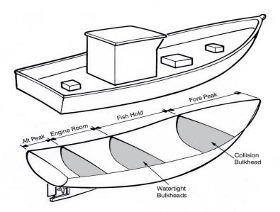
Leaks in the engine room are often caused by a corroded seacock, damaged seawater hoses, poor quality and installation of wet exhaust hose and a faulty stuffing box in the stem tube. If the buoyancy of the aft peak is sufficient, the boat will float. A collision with a boat, a log or a rock could lead to flooding of the boat. A forward watertight bulkhead will prevent flooding of the whole boat.
