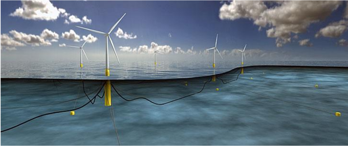
Figure 5: Schematic of Completed Hywind Pilot project
