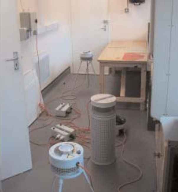
SUPERfume system set up in a small laboratory at PSDB Sandridge
