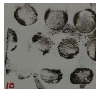
Figure 17: Light footwear mark treated with (a) acid black 1, then (b) iron oxide powder suspension.
