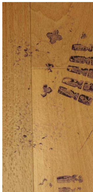
Figure 18: Footwear mark in blood on lino flooring treated with acid violet 17 followed by iron oxide powder suspension
