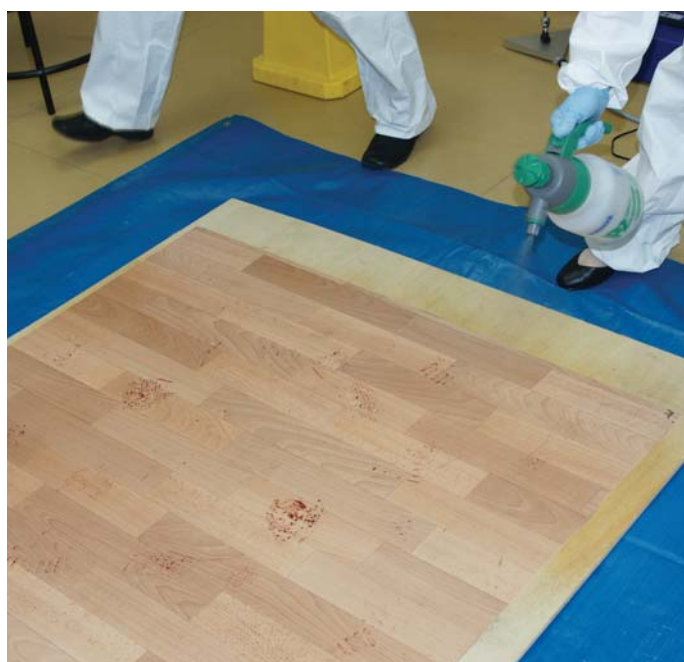
Figure 14: Trial 2. The flooring surface was fixed by spraying the fix solution with a garden spray and leaving for 30 minutes.
