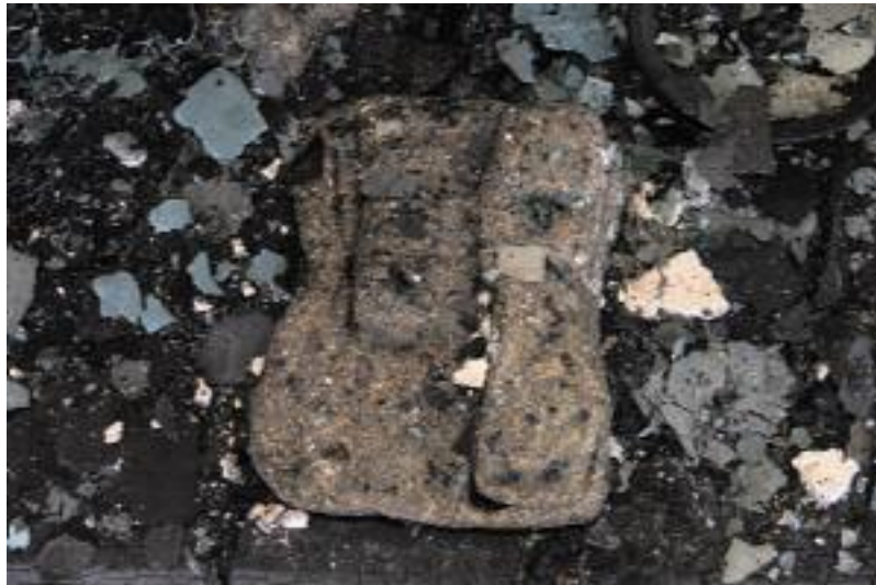
Upper surface of telephone exposed to fire scene, showing melting and heavy soot coverage (photograph reproduced courtesy of Gardiner Associates)
