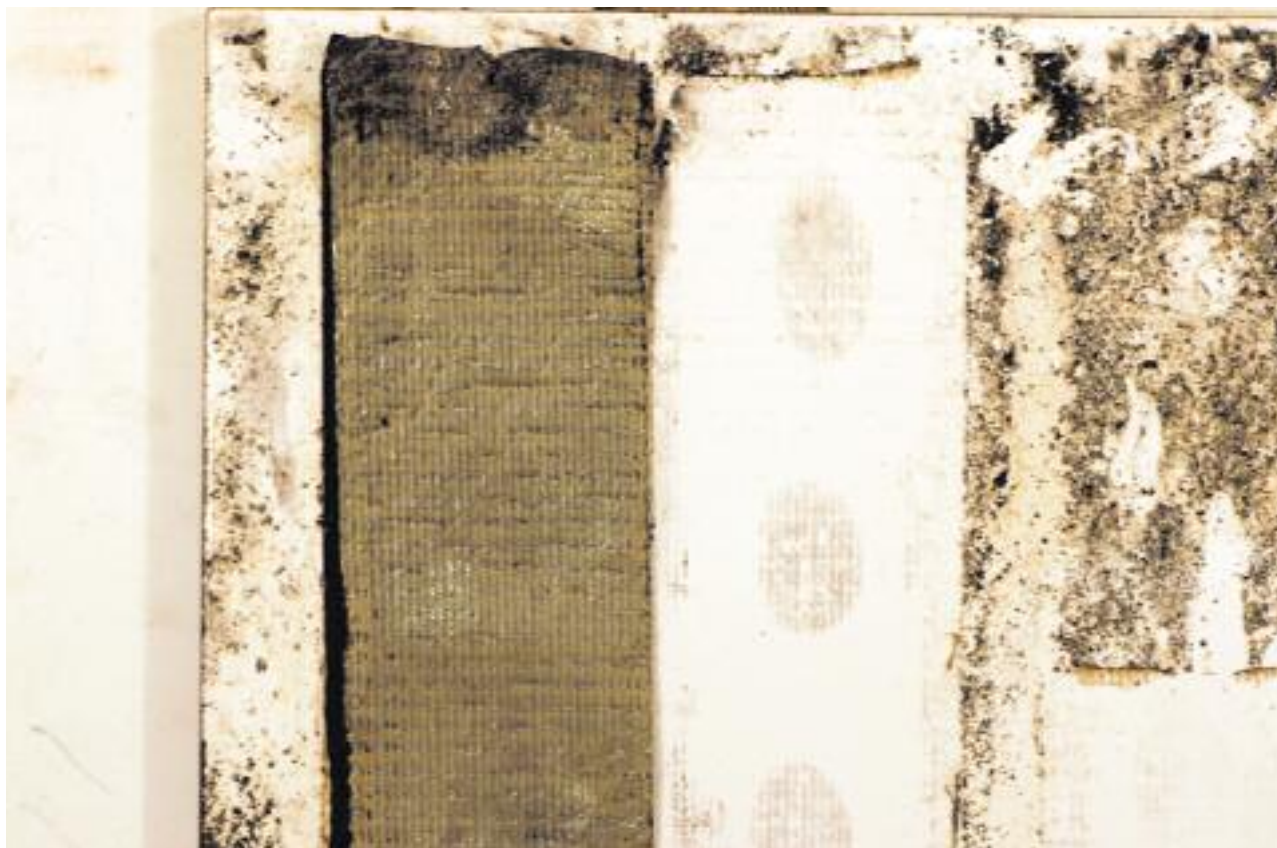
Development of fingerprints on adhesive tapes using black powder suspension. Weak development on adhesive side, stronger development of reversed mark on ceramic tile substrate.
