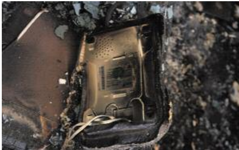
Underside of telephone, showing that protected surface is relatively undamaged and more likely to yield marks. (photograph reproduced courtesy of Gardiner Associates)
