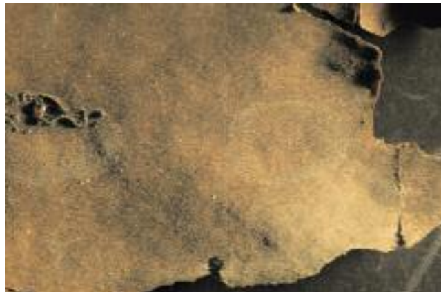
Fingerprints developed on charred region of paper exhibit using Physical Developer.
