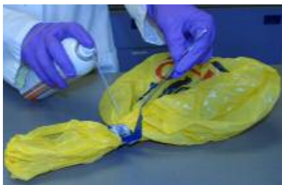
Removal of tape from a polythene bag with freezer spray
