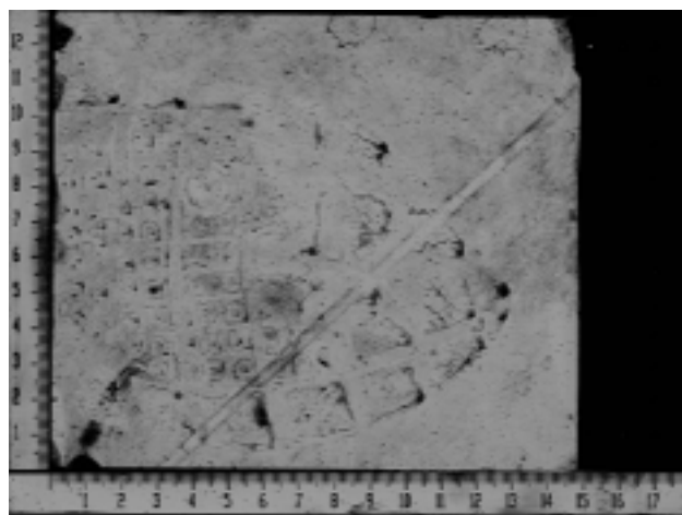
Reverse image of a dusty footwear mark lifted from lino flooring with a black gel-lifter and imaged using the BVDA GLScan.
