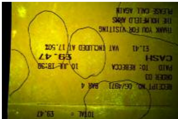
Areas of ridge detail on a thermal receipt processed using DMAC
