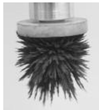
Figure 11: Magnetic applicator loaded with black magnetic powder
