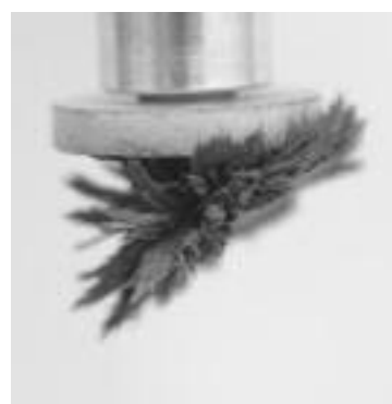
Figure 13: Magnetic applicator loaded with magnetic grey powder
