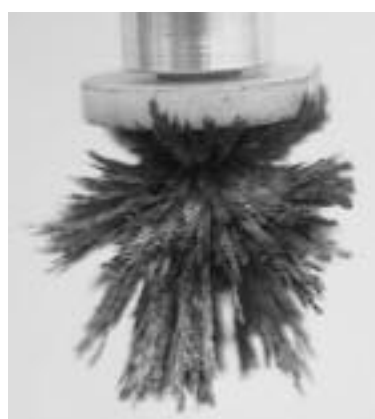
Figure 12: Magnetic applicator loaded with magneta flake
