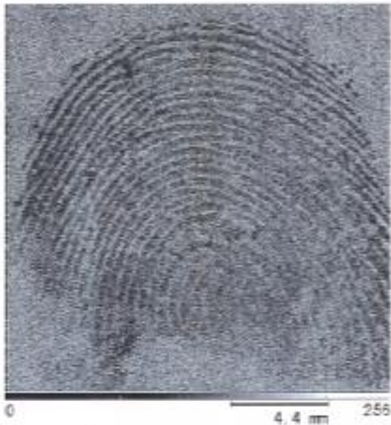
XRF microscope image of iodide toned PD mark using x-ray transmission mode
