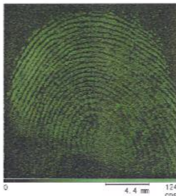
XRF microscope image from iodine X-ray fluorescence
