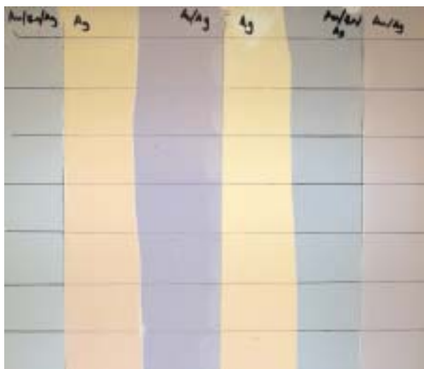
Strips of freezer bag treated with different VMD metal combinations
