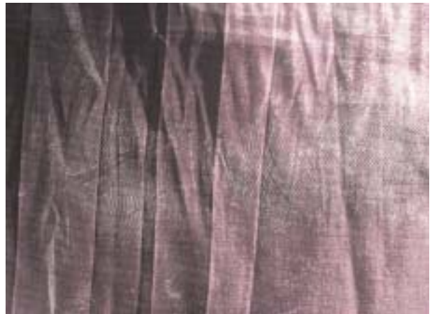
Mark developed on fine-weave polyester fabric using superglue.
