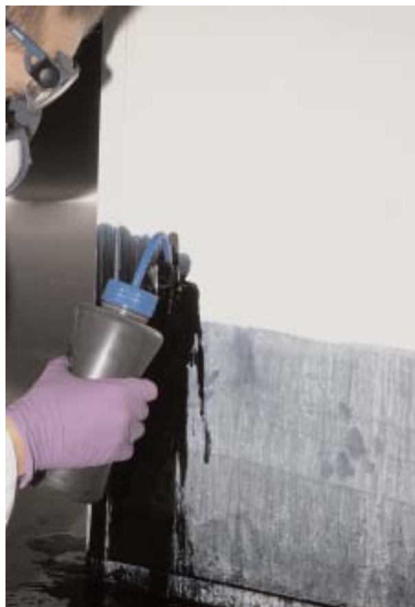
Treatment of surface with Solvent Black 3 working solution
