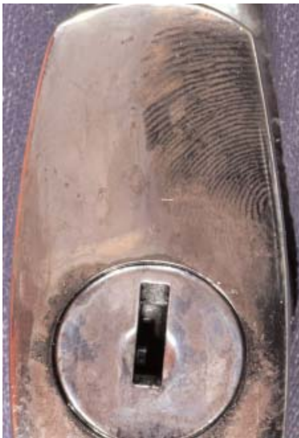
Fingerprint developed with Solvent Black 3 on a door lock
