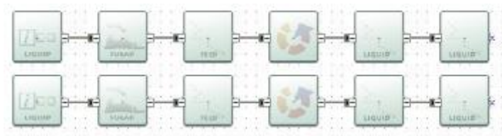
Figure 26 Correct representation of parallel streams in a fuel chain
