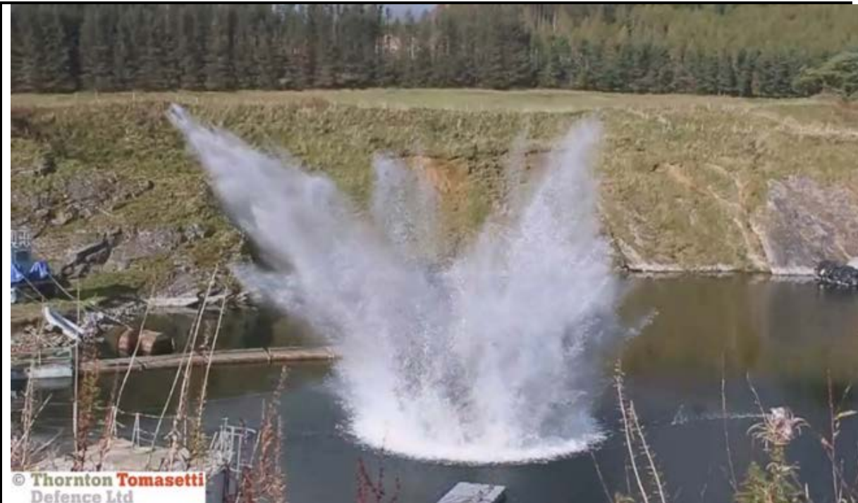
Figure 4-5 A 10 kg high-order detonation at the quarry site (courtesy of Thornton Tomasetti Defence Ltd)
