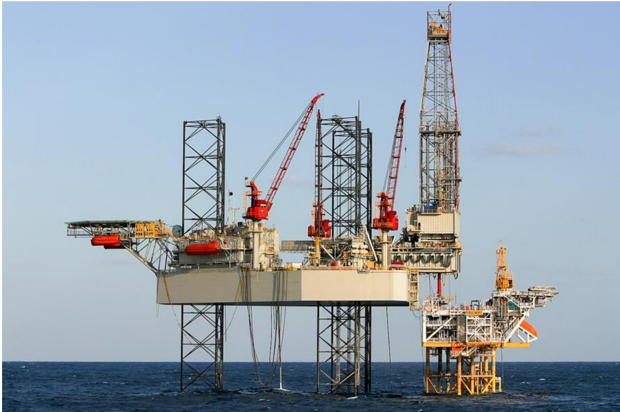
Figure 3.2 – Typical jack-up rig (e.g. shown is the Ensco 104) over a small platform
