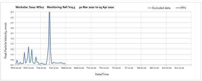
Note: High vibration levels measured at 08:00 on Tuesday 31st March were due to local disturbance of the vibration monitor and are not representative of HS2 vibration levels.
