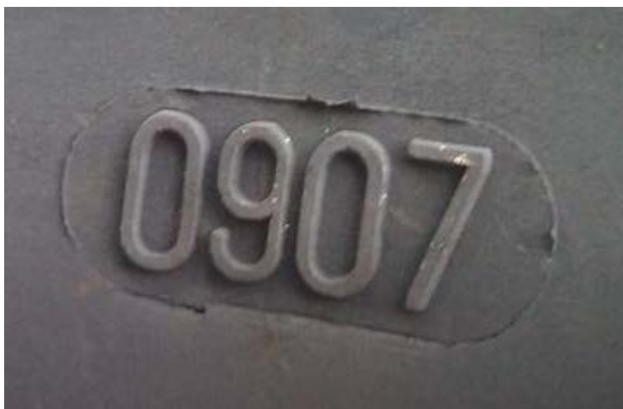
Image 1: Example tyre date stamp on the side wall of a tyre
