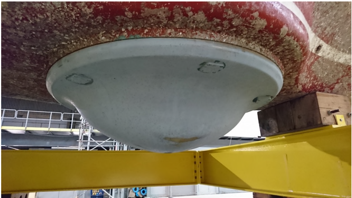
Sonar transit dome in place.
