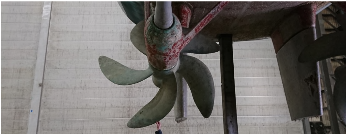
Starboard propeller – since removed and stowed on upper deck.
