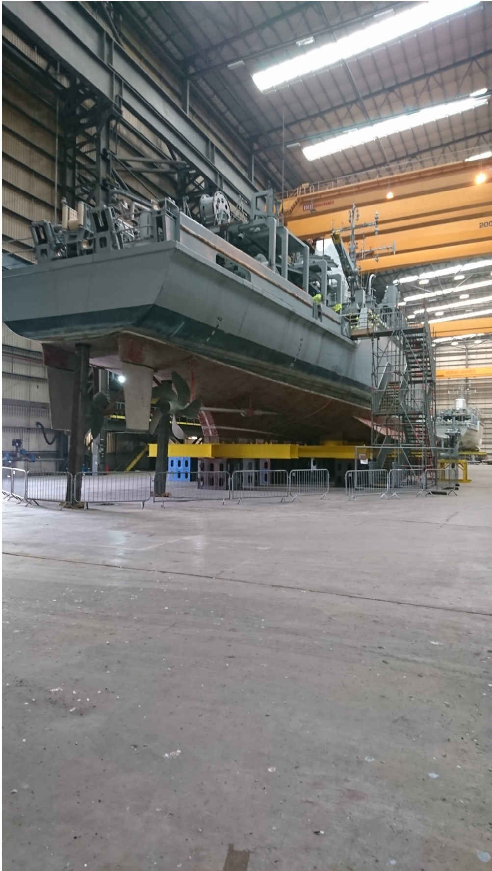
Starboard Quarter view: Props removed and stowed on upper deck, shaft glands sealed.
