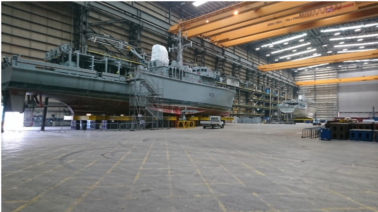
Starboard side view: props removed and stowed on upper deck, shaft glands sealed.
