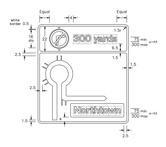
This drawing should be used in conjunction with the Traffic Signs Manual Chapter 7
