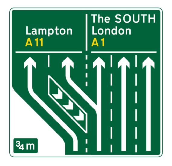
Aside from the colours, all the dimensions required to design this sign are the same as shown on working drawing Schedule 12 Part 28 Item 02 (P2904.2).
