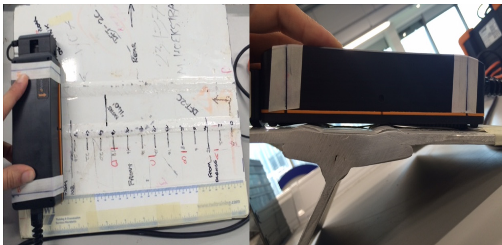
Figure 10 Top view and side view of the circumferential weld (showing the lift-off).
