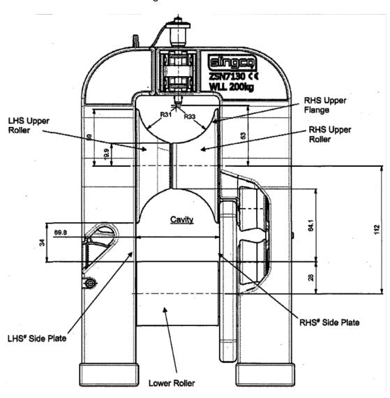
12. The Catch Block is said to include an upper roller assembly formed from a left roller and a right roller together with a flat lower roller having a substantially constant cross sectional diameter. There is a substantial 34mm gap between the lower roller and the flanges of the upper rollers. In order to emphasise that this gap is substantial the request explains that it is not small enough to prevent the conductor from touching side plates of the Catch Block.
