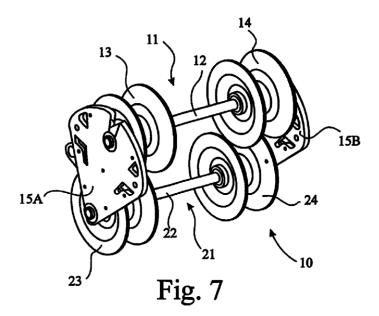
6. In use the upper rollers 11 can be released from the lower rollers 21 in order that a conductor can be placed in each cavity defined between the flanges of the upper and lower roller pairs as the upper rollers 11 are replaced. Each roller assembly 10 is connected in use to adjacent roller assemblies 10 by means of straps 20, the end of one of which is shown in figure 11.
