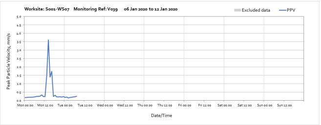
Note: Missing data between 08:00 on Tuesday 7<sup>th</sup> January and 15:00 on Wednesday 29<sup>th</sup> January was due to the removal and reinstation of the vibration monitor on site due to vehicles accessing the site within close promixity to the monitor.
