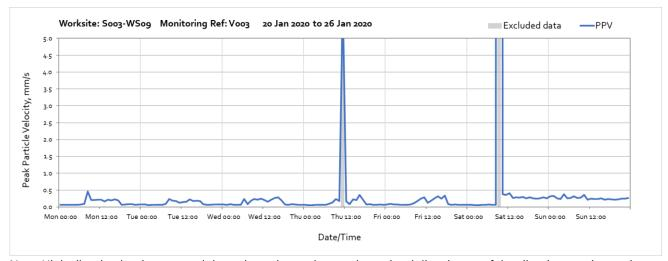
Note: High vibration levels measured throughout the week were due to local disturbance of the vibration monitor and are not representative of HS2 vibration levels.
