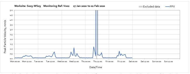
Note: High vibration levels measured at 11:00 on Thursday 30<sup>th</sup> January were due to local disturbance of the vibration monitor whilst the monitor battery was changed and are not representative of HS2 vibration levels.
