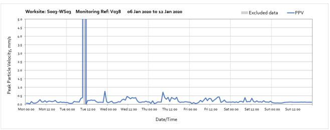
Note: High vibration levels measured at 10:00 - 11:00 on Tuesday 7<sup>th</sup> January were due to local disturbance of the vibration monitor during routine maintenance of the monitor and are not representative of HS2 vibration levels.
