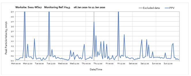
Note: High vibration levels throughout the week were due to local disturbance of the vibration monitor and are not representative of HS2 vibration levels.
