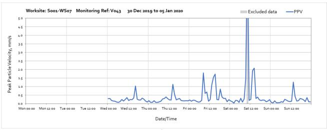
Note: High vibration levels measured at 10:00 on Saturday 4<sup>th</sup> January were due to local disturbance of the vibration monitor and are not representative of HS2 vibration levels.
