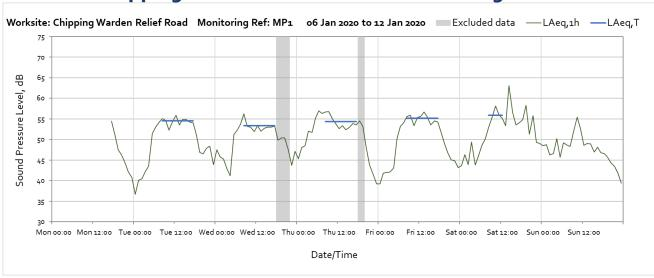
Note: Missing data until 17:00 on the 6<sup>th</sup> of January were due to an equipment failure.
