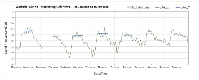
Note: Missing data between 02:00 and 12:00 on Tuesday 21st of January was due to loss of external power to the monitoring station.
