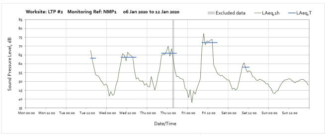
Note: Missing data between the start of the month and 14:00 on Tuesday 7<sup>th</sup> January was due to loss of external power to the noise monitor.
