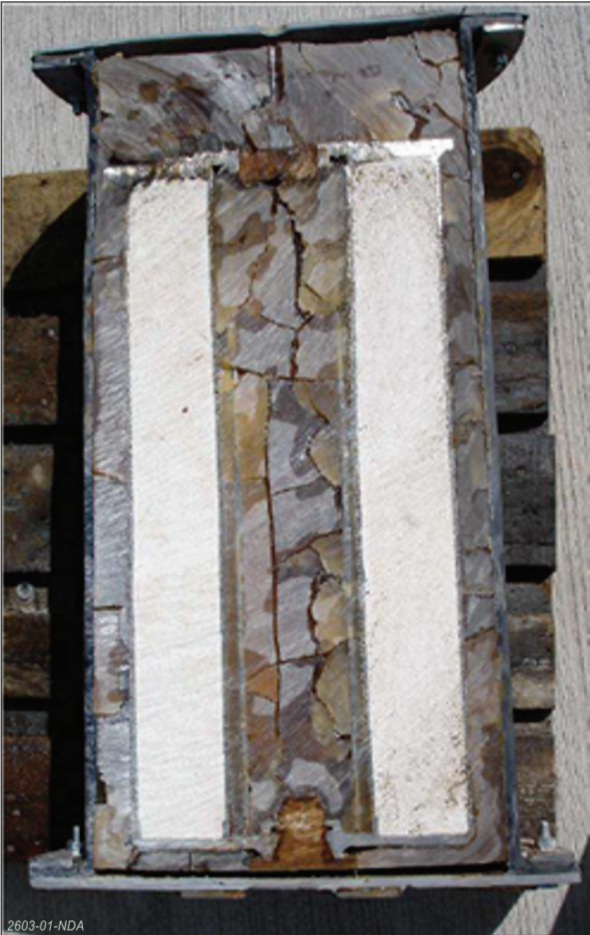
Figure 8 Sectioned product showing cracking in cured resin
