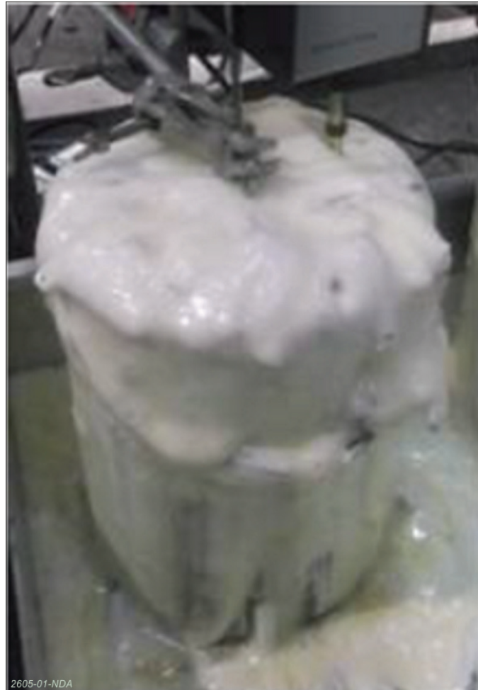
Figure 10 Foaming observed during epoxy resin encapsulation of aluminium and CMS
