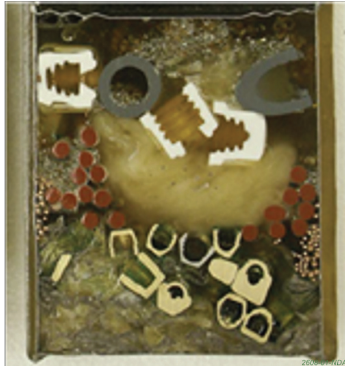
Figure 13 Sectioned can of simulated radium bearing wastes infilled with polyester resin
