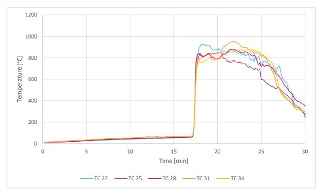
Figure G42 – Temperatures measured on the cavity central axis for S24
