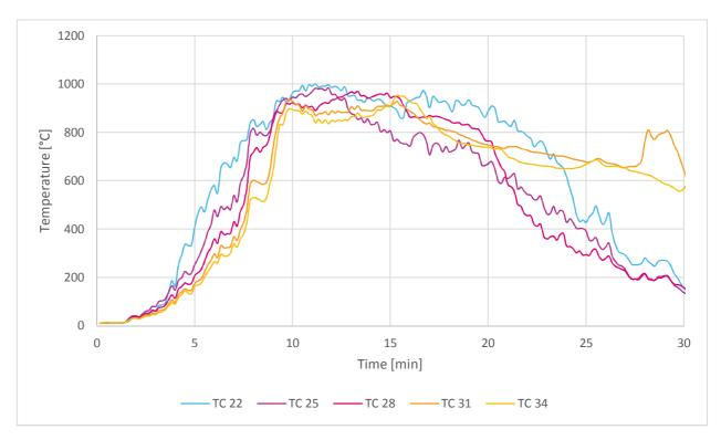
Figure G46 – Temperatures measured on the cavity central axis for S26
