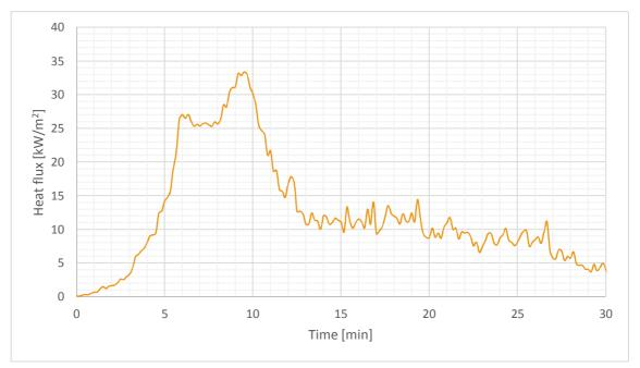
Figure G14 – Heat flux recorded during the fire at 3.0 m height
