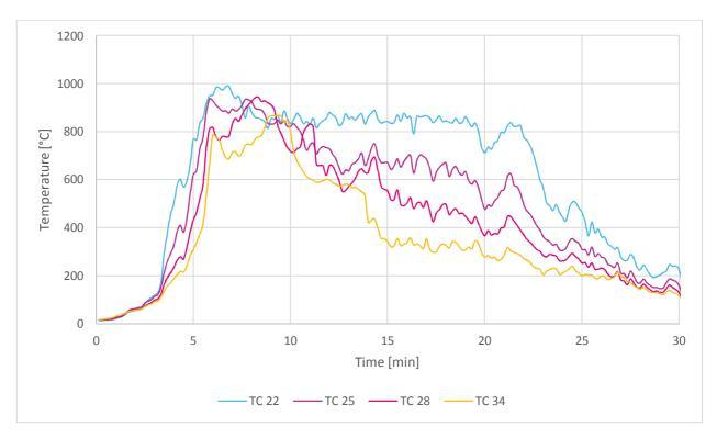
Figure G44 – Temperatures measured on the cavity central axis for S25
