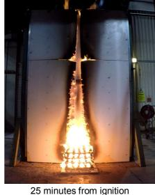
Figure G17 – Photographs during the fire at 5, 10, 20, and 25 minutes from ignition
