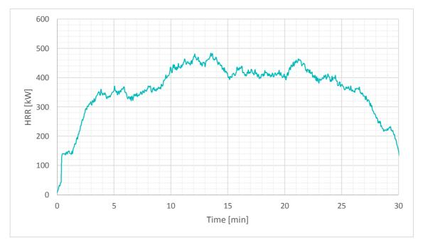
Figure G18 – Heat release rate measured during the fire, including the source
