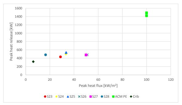
Figure G36 – Results related to measured peak heat release rate and measured peak heat flux including PE ACM panels used for calibration
