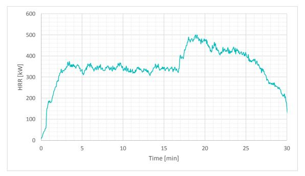
Figure G8 – Heat release rate measured during the fire, including the source
