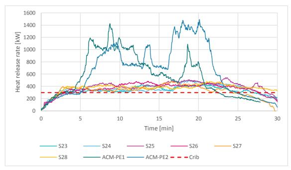
Figure G32 – Heat release rate for all samples showing base value of ignition source and comparison with PE ACM samples
