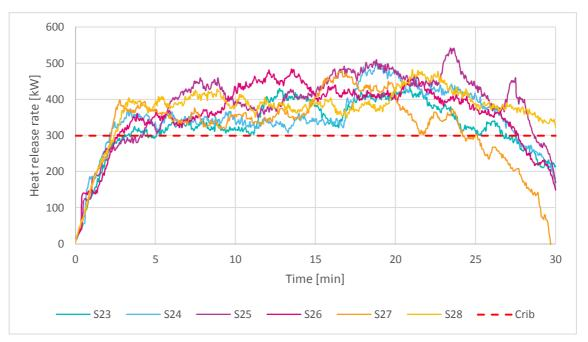
Figure G31 – Heat release rate for all samples showing base value of crib
