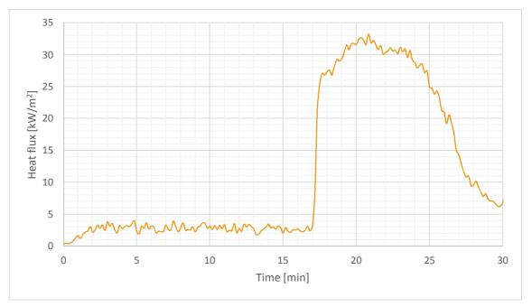
Figure G9 – Heat flux recorded during the fire at 3.0 m height
