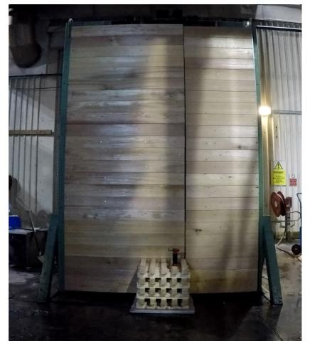
Figure G26 – Sample S28 timber cladding installed on the rig
