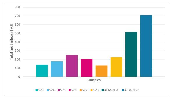
Figure G33 – Total heat release for all samples compared with PE ACM samples
