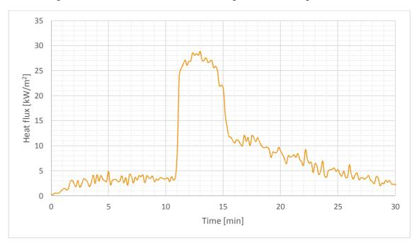
Figure G4 – Heat flux recorded during the fire at 3.0 m height
