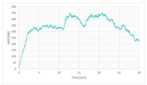
Figure G3 – Heat release rate measured during the fire, including the fire source
