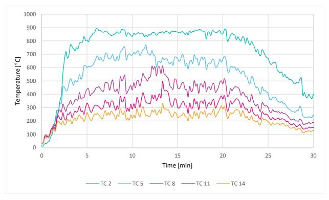
Figure G39 – Temperatures measured on the external central axis for S23
