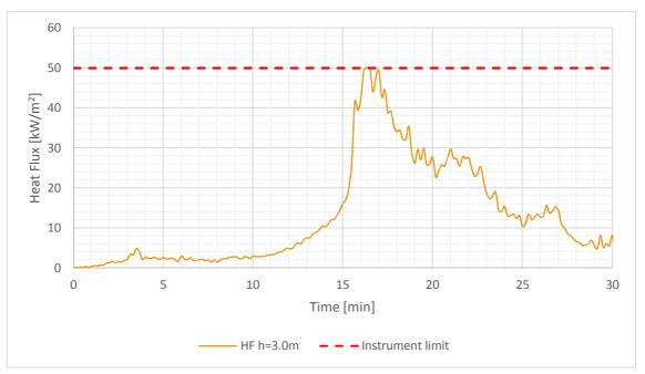
Figure G24 – Heat flux recorded during the fire at 3.0 m height
