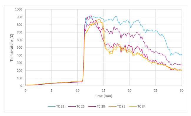
Figure G40 – Temperatures measured on the cavity central axis for S23
