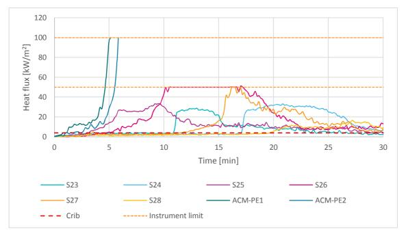
Figure G35 – Measured heat flux for all samples at 3 m from the ground on the centre line
