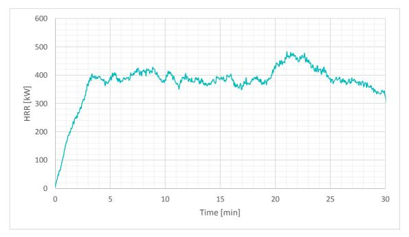
Figure G28 - Heat release rate measured during the fire, including the source
