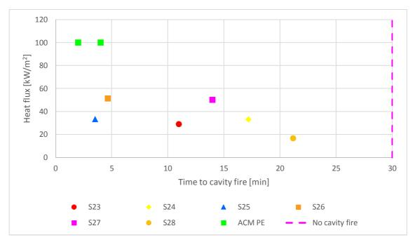
Figure G37 – Comparison of measured peak heat flux and time to burn through of the panels
