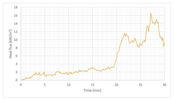
Figure G29 – Heat flux recorded during the fire at 3.0 m height
