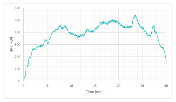
Figure G13 - Heat release rate measured during the fire, including the source
