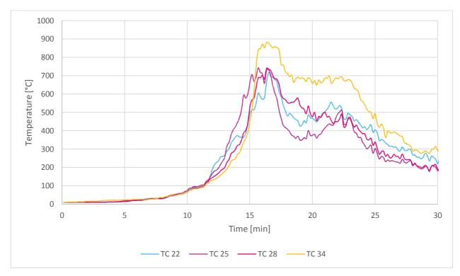
Figure G48 – Temperatures measured on the cavity central axis for S27
