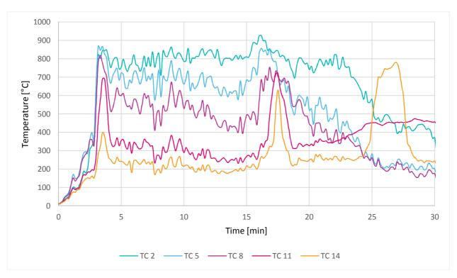
Figure G47 – Temperatures measured on the external central axis for S27
