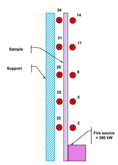
Figure G38 – Thermocouple locations for the samples
