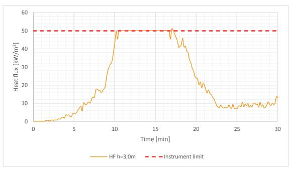
Figure G19 – Heat flux recorded during the fire at 3.0 m height
