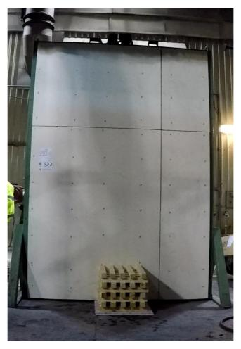
Figure G6 – Sample S24 HPL panels installed on the rig
