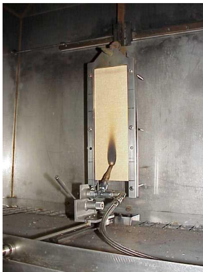
Figure A11 – Small flame test apparatus [27]
