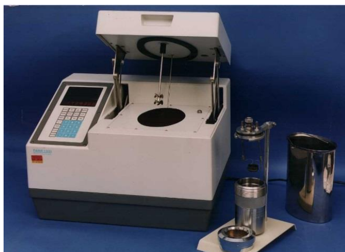
Figure A10 – Test apparatus for bomb calorimetry [26]
