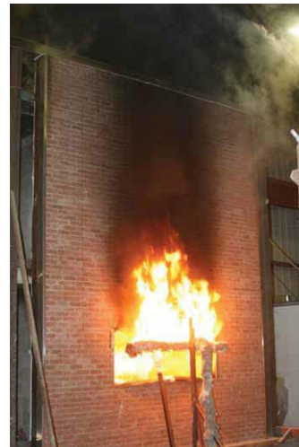
Figure A20 – NFPA 285 test apparatus front view without test wall (left) and during a test (right) [53]
