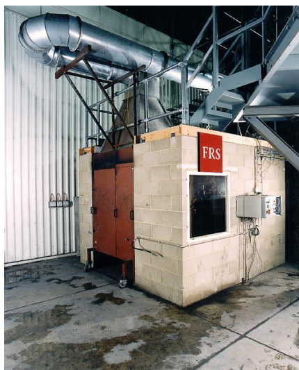
Figure A12 – Single Burning Item test – external view [28]
