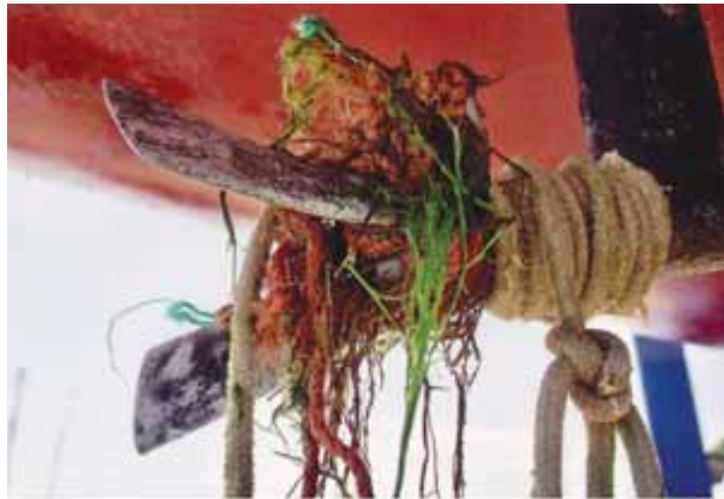
Folding prop with entangled rope
