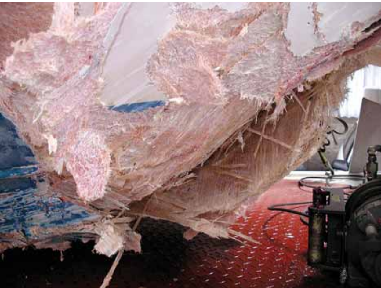
Figure 2 – Damage to starboard forefoot and bow forward
