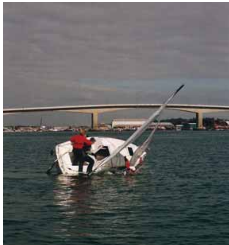
Figure 2 – Test report photograph – small trailer-sailer being capsized
