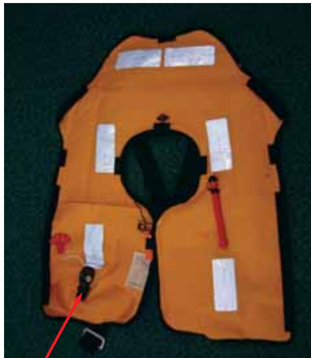
CO 2 bottle missing
