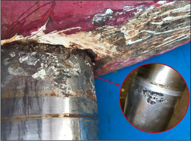
Figure 2: The rudder stock of the sister yacht, showing pitting and evidence of corrosion
