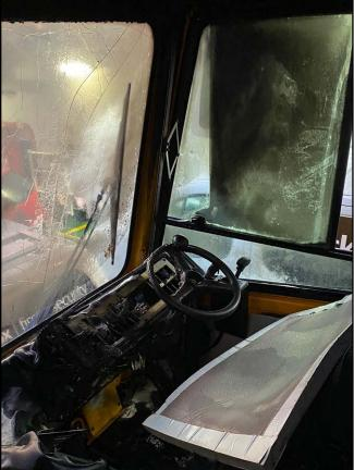
Figure 2: Fire damage to the cab of the tug master after the fire had been extinguished
