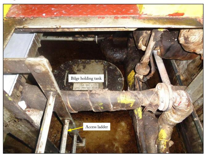
Figure 1: Access to bilge holding tank manhole cover
