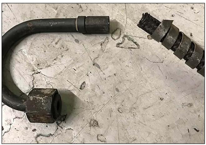
Figure 1: The failed turbocharger oil feed pipe
