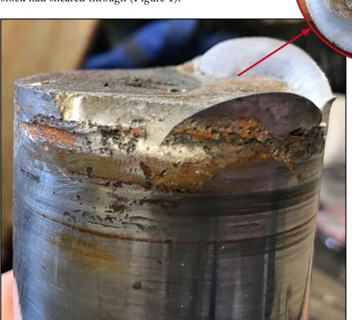
Figure 1: The failed rudder stock showing the effects of crevice corrosion
