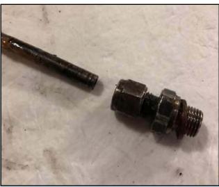
Figure: The failed compression fitting (olive not shown)
