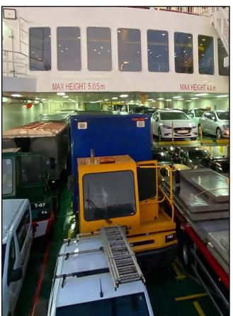
Figure 1: The tug master unit and lorry trailer on board the ferry
