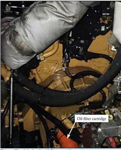
Figure: Clutch hydraulic oil filter cartridge
