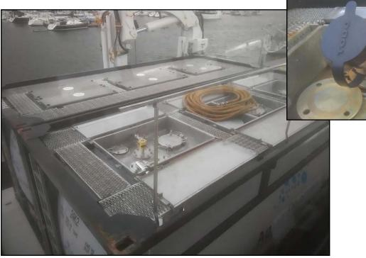
Figure: The hydrogen peroxide tanks as seen from the wheelhouse (inset: the valve being removed)
