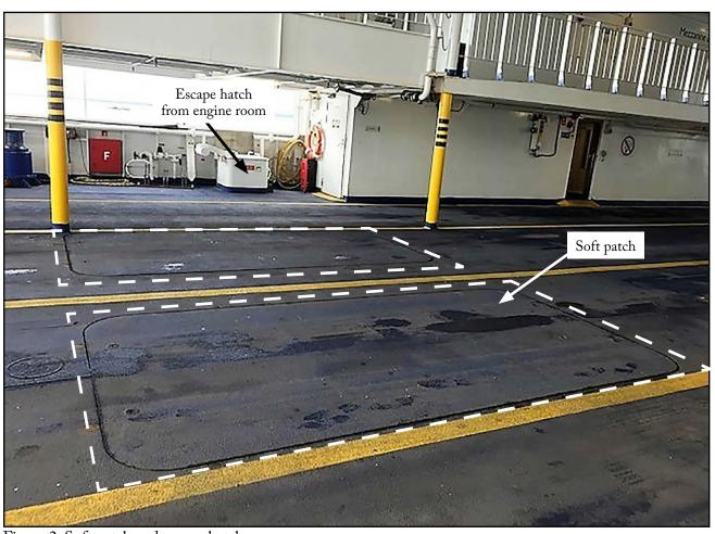
Figure 2: Soft patch and escape hatch
