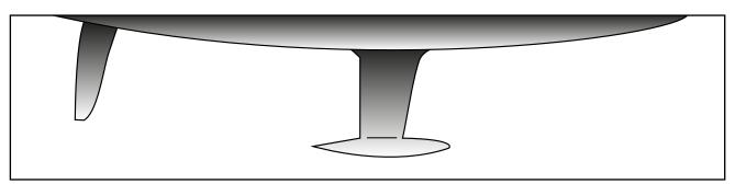
Figure: Modern keel and rudder arrangements are efficient but potentially vulnerable and should be professionally examined following a grounding
