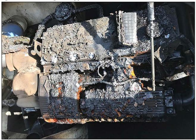
Figure 2: Fire damage to the port main engine and its compartment
