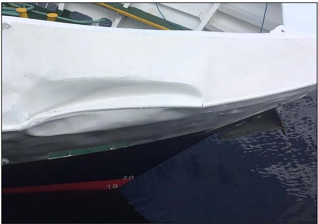
Figure: Structural damage to the ferry's starboard bow after the impact
