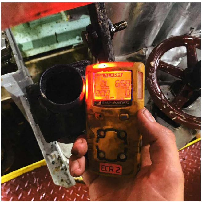
Figure 2: Multi-gas meter readings immediately after the incident
