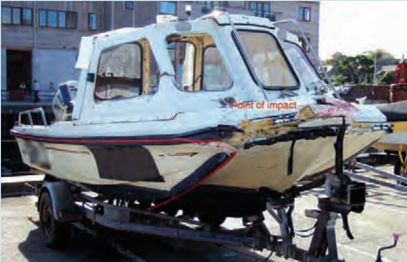
Figure 3: Damage to bow of the dory
