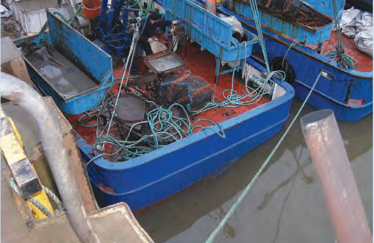
Figure 2: View of stern showing limited freeboard
