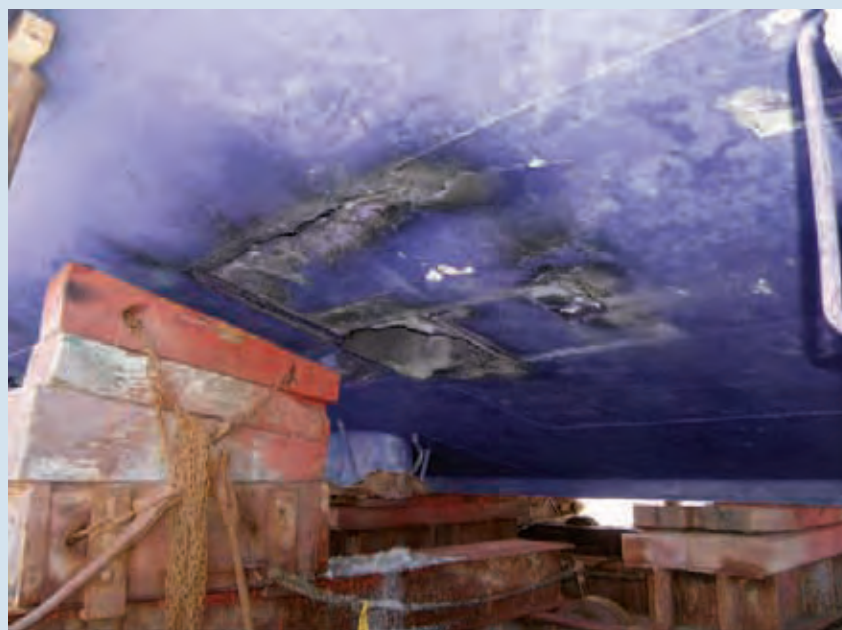
Some of the damage caused by the grounding
