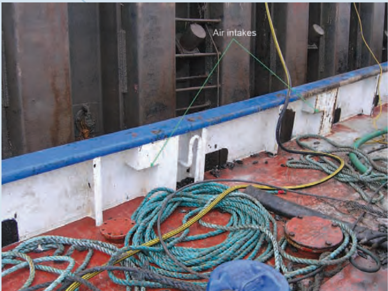
Figure 1: Deck, showing engine room air intakes
