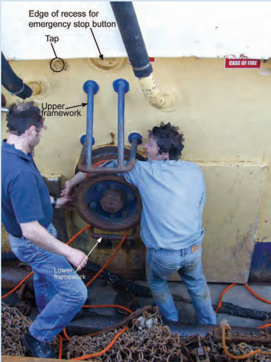
Figure 2: Demonstration of "as-found" position of deckhand, trapped in whipping drum
