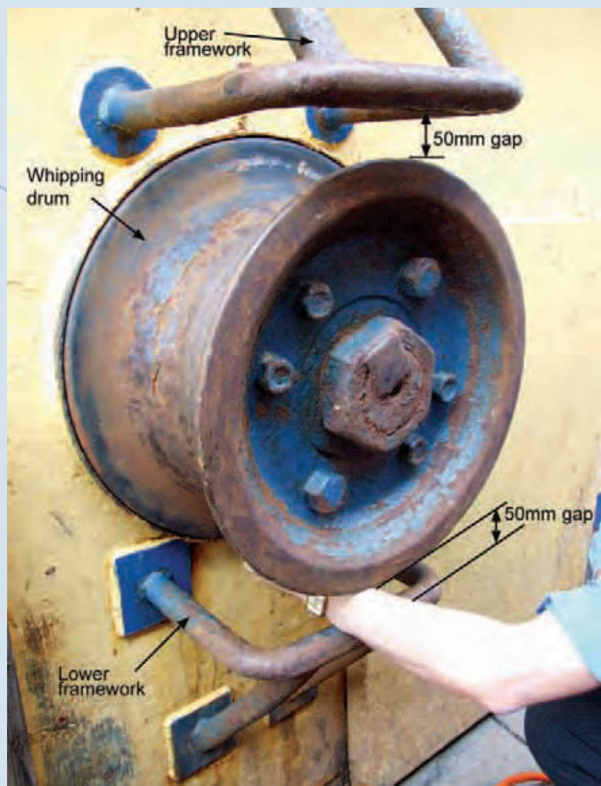
Figure 1: Port whipping drum with demonstration of an arm in the gap between winch head and lower framework
