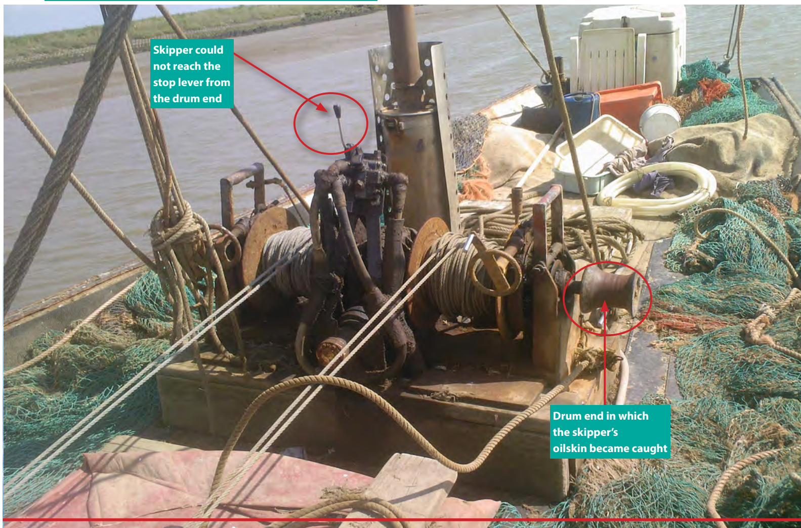
Figure 22*: View of the working deck where the accident occurred
