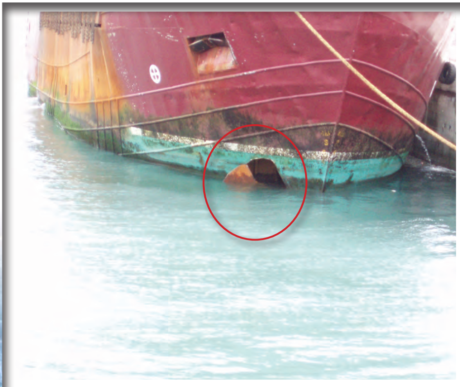
Figure 24: Shell plating damage
