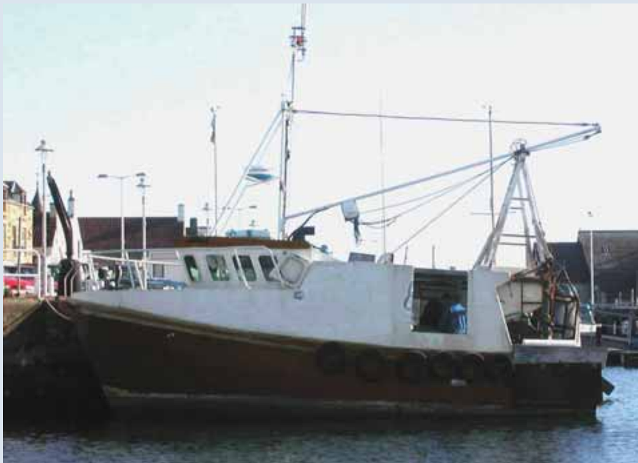
Photograph showing the vessel's point of suspension for the dog rope and cod end
