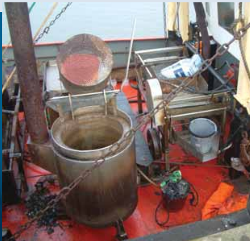
Figure 2: Shrimp boiler after the fire, with melted air supply pipe
