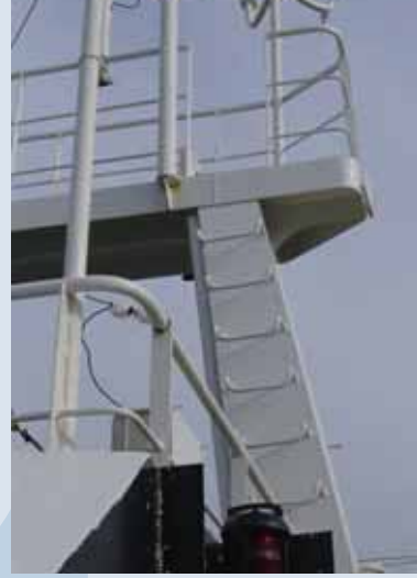
Figure 2: Port ladder and access showing unguarded gap.
