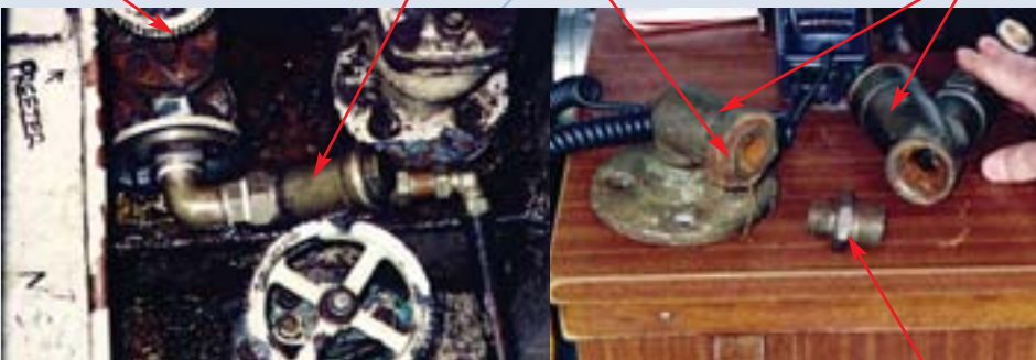
Example pipe fitting – showing design of failed item
