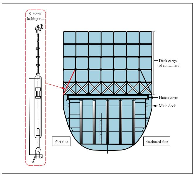
Figure: Diagram of ship viewed from aft to forward, indicating location of lashing rod
