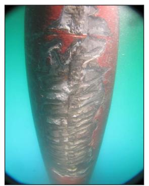
Figure 1: Damage to port rudder
