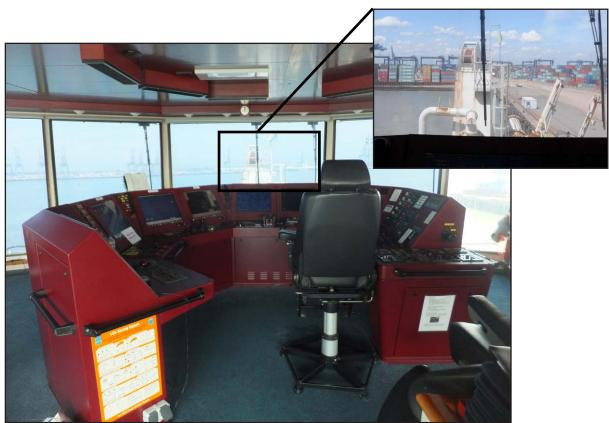
Figure 2: Bridge conning position (inset: obstruction)
