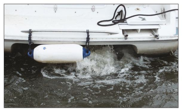
Figure 2: Wet exhaust at boat's stern
