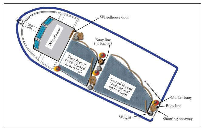
Figure 2: Storage of two fleets of creels on deck of fishing vessel (as on the day of the accident)
