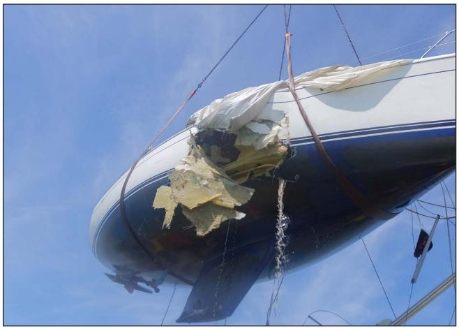
Figure 3: Damage to starboard side of yacht
