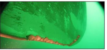
Figure 2: Damage to starboard propeller tip
