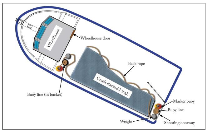
Figure 1: Single fleet storage of creels on deck of fishing vessel
