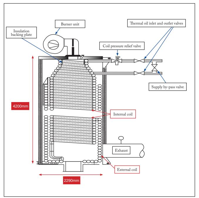
Figure 1: Diagram of the port thermal oil heater
