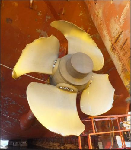
Figure 1: The damaged port propeller
