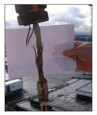
The fall wires had been fitted on board the ferry for almost 4 years and had been maintained, greased and inspected in accordance with company and onboard instructions throughout. The grease used was black. No issues relating to the condition of the wires had been recorded.
