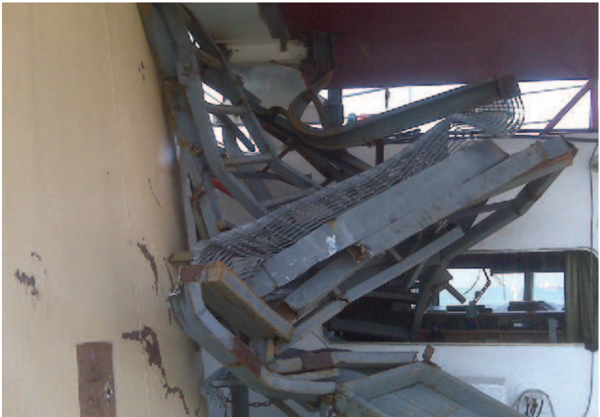
Figure 2: Damage to the container gantry jib
