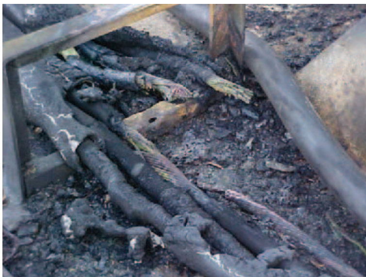
Figure 4: Close-up of the damaged cables
