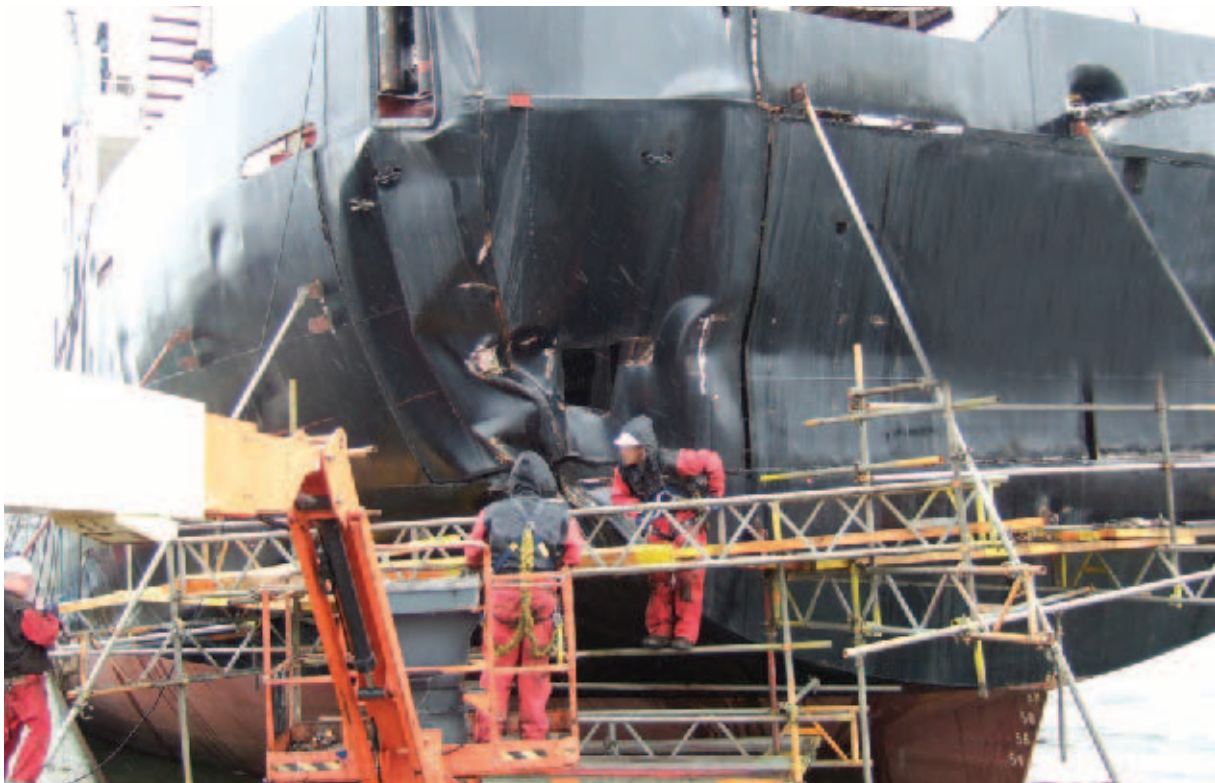
Figure 1: Damage sustained to stern of vessel
