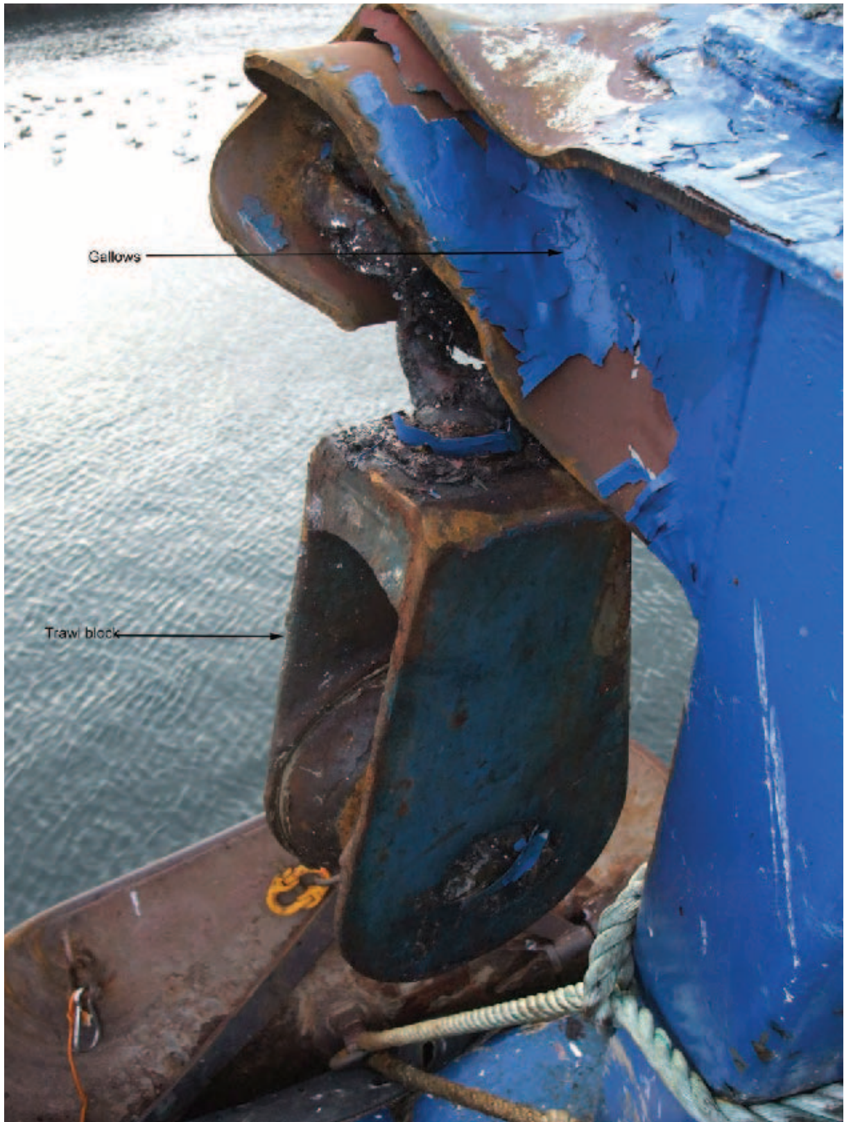
Figure 2: Damage sustained to gallows and trawl block of fishing vessel
