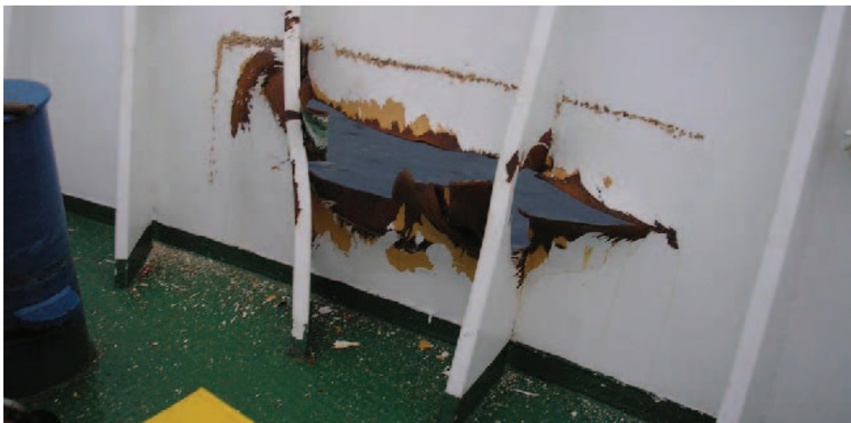
Figure 1: Damage sustained to port bow bulwark on cargo vessel
