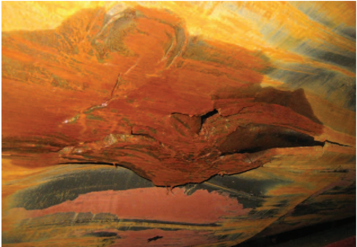
Figure 2: The extent of the hull penetration
