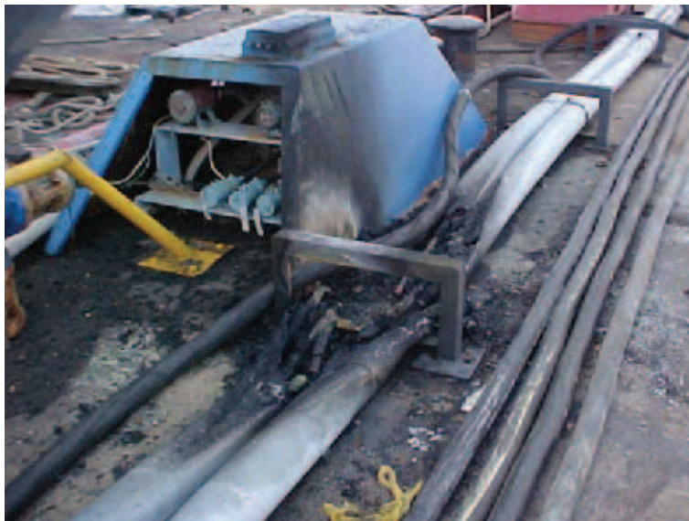
Figure 3: Damage to the supply lines
