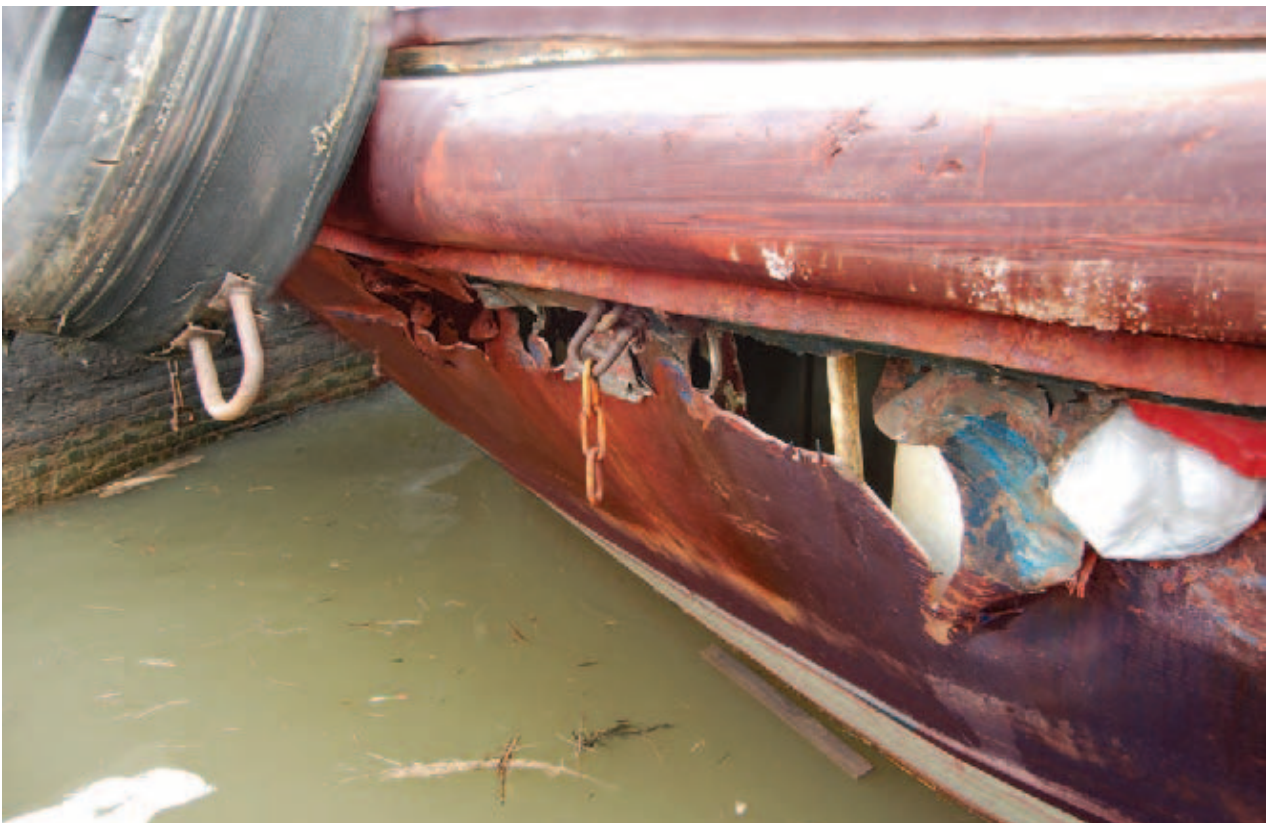
Figure 3: The damage sustained to the tug
