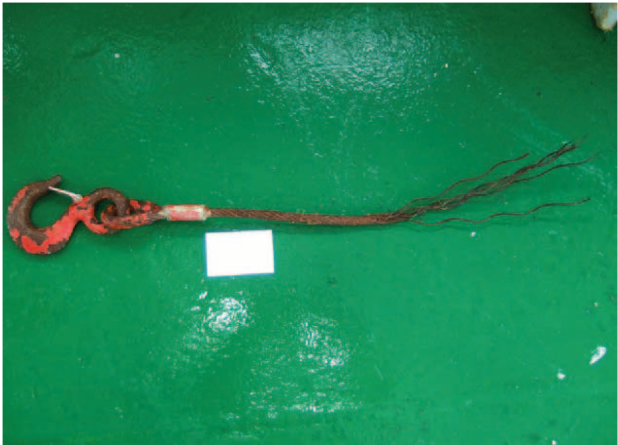
Figure 2: Stores davit hook and parted wire
