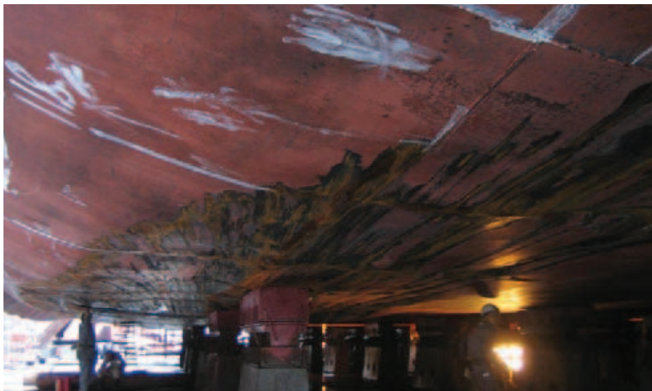
Figure 1: Damage sustained to the hull of the vessel
