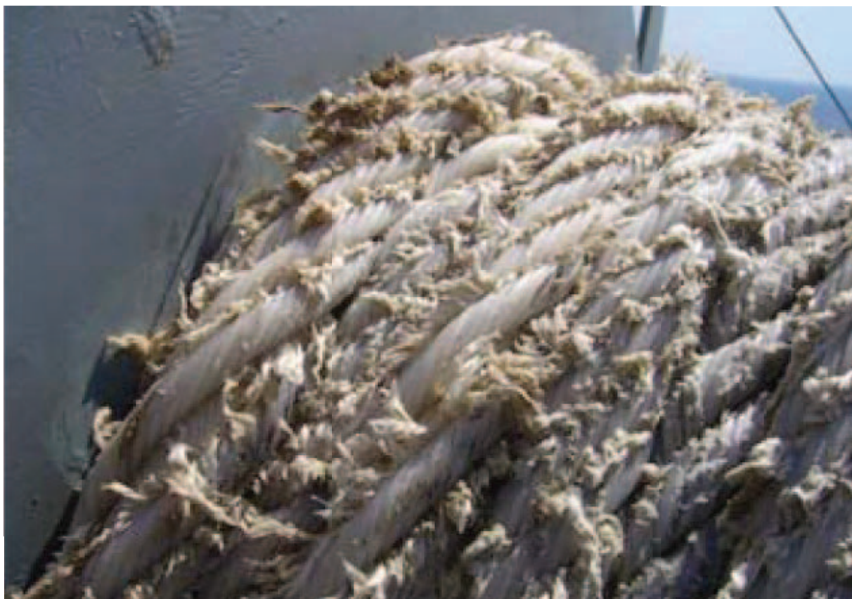
Figure 3: The mooring lines were in poor condition
