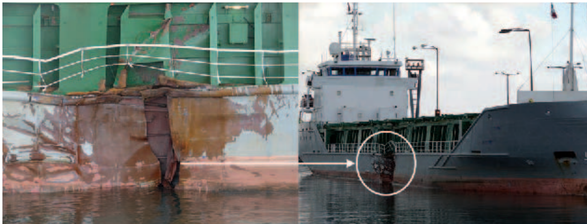
Figure 2: Damage sustained to starboard side of general cargo vessel
