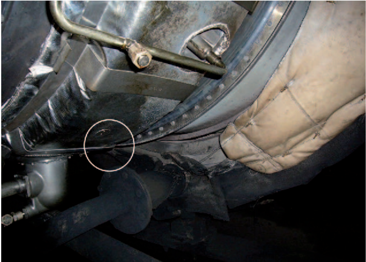
Figure 2: Position of plenum seal leak
