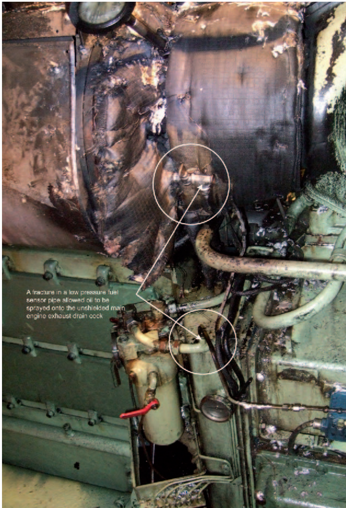
Detail showing diesel oil filter, pressure alarm and unshielded drain cock
