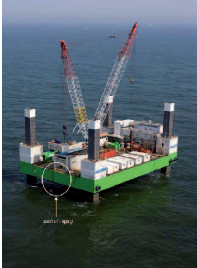
Figure 2: Jack up barge - point of impact
