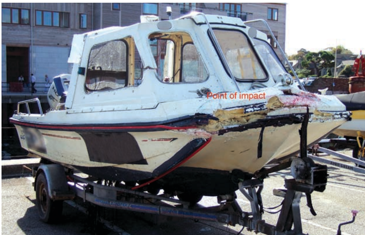
Figure 3: Damage to bow of the dory
