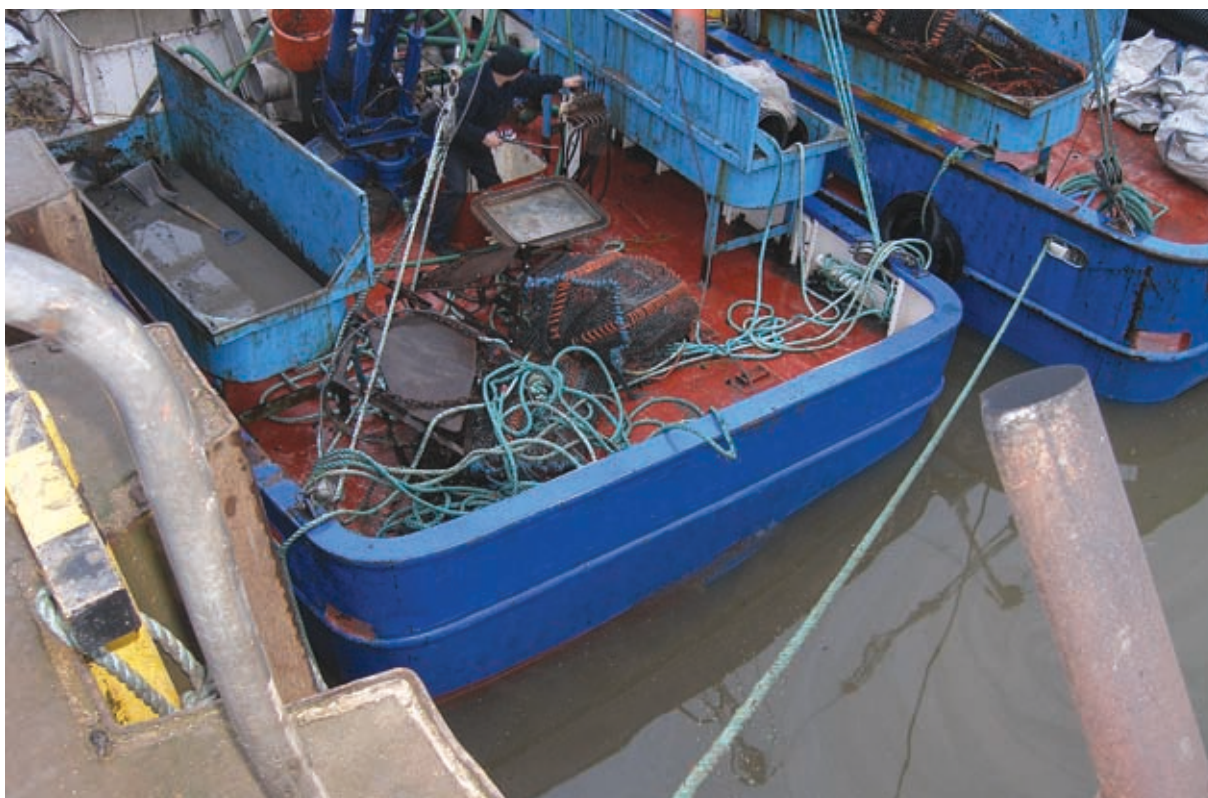
Figure 2: View of stern showing limited freeboard
