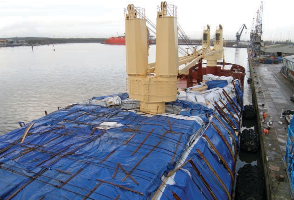
Figure 2: View forward, showing damaged uprights
