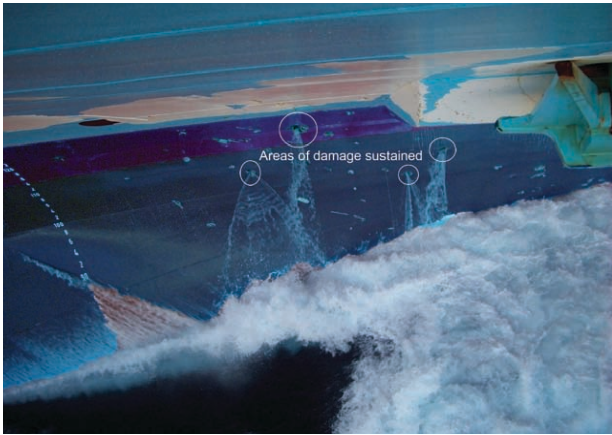
Figure 2: Hull holes and indentations
