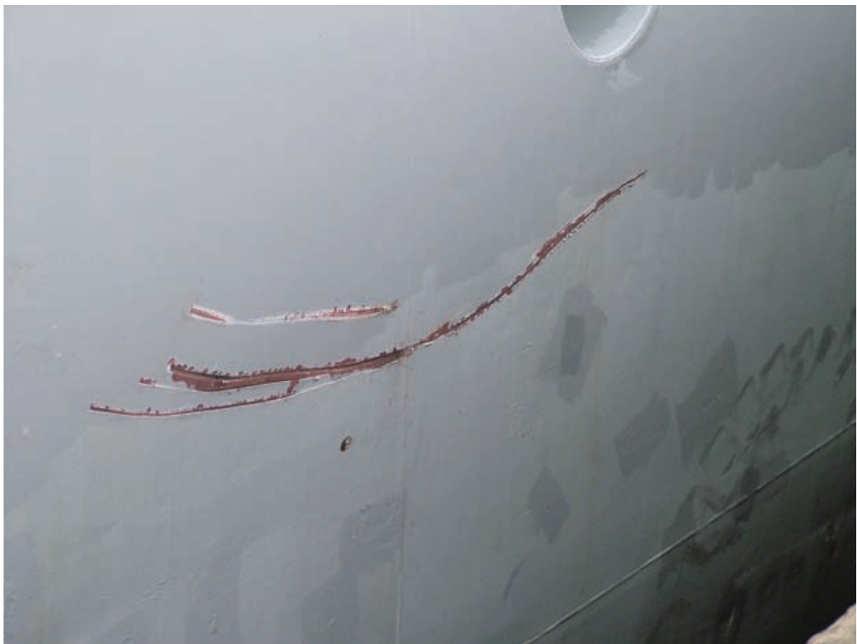
Figure 1: Damage to merchant vessel caused by contact with the derrick on the fishing vessel
