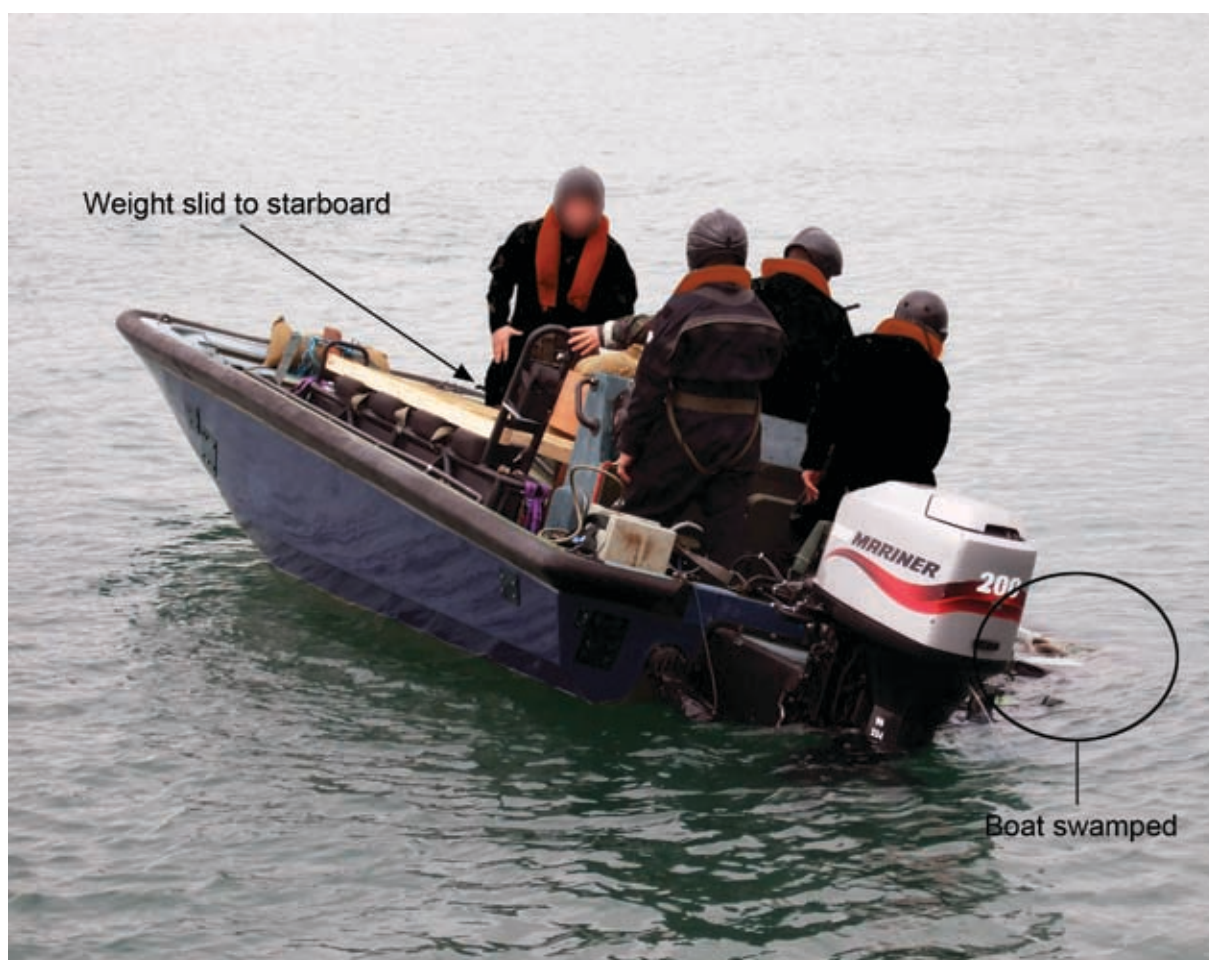
Capsize trial illustrating weight shift and boat swamping
