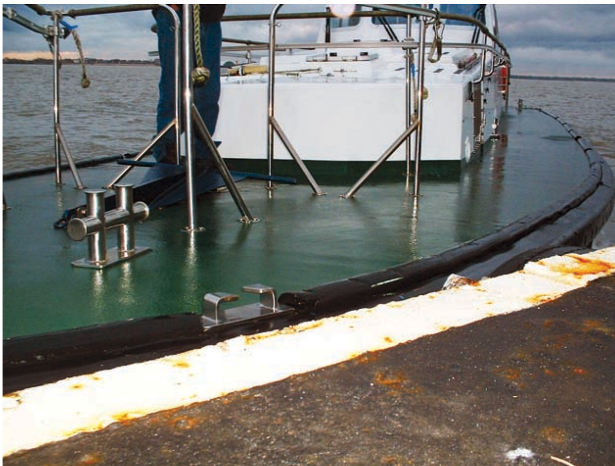
Figure 1: Pilot boat with port shoulder leaning against tyre fender of pontoon
