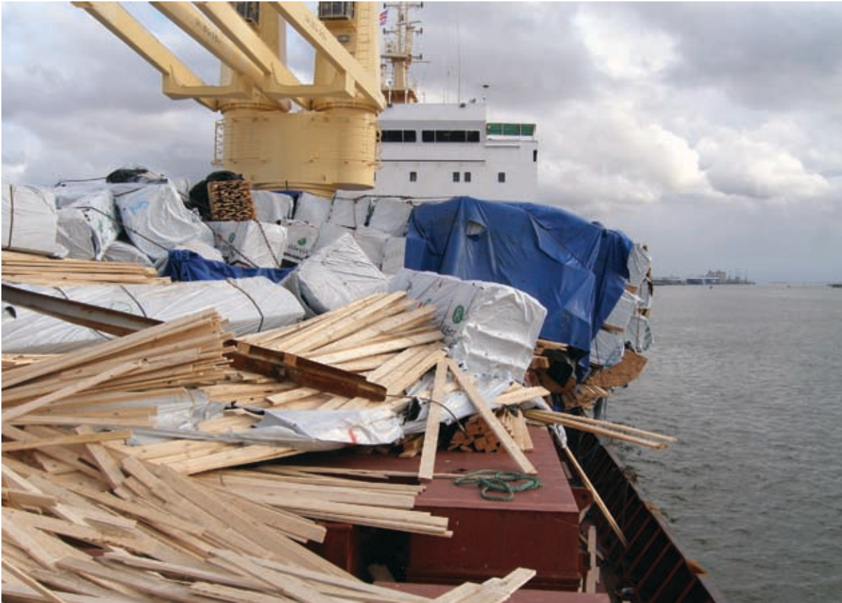
Figure 1: Port side – showing collapsed stow. Note the smooth surface on the hatch covers
