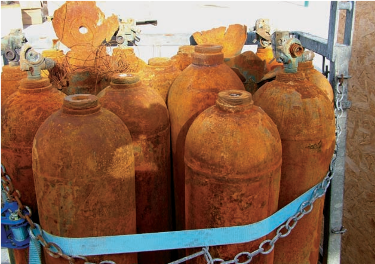
Figure 4: Acetylene bottle damage
