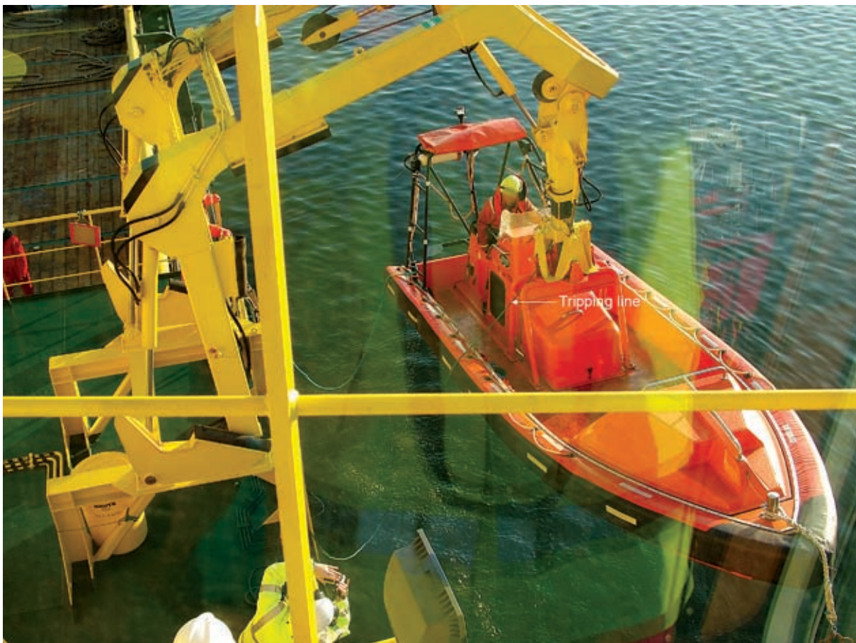
Fast Rescue Craft securing arrangement
