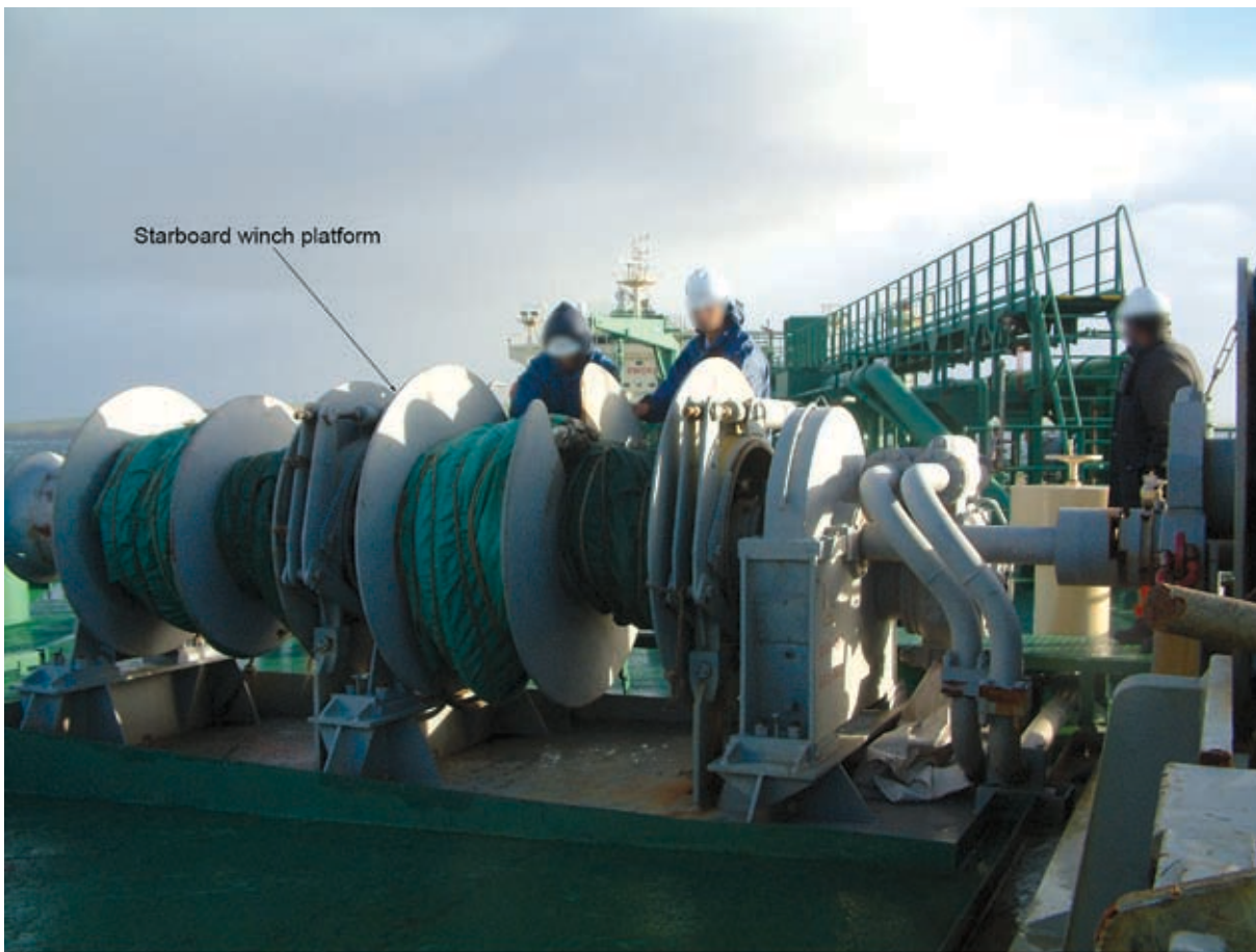
Position of crew at the starboard winch platform
