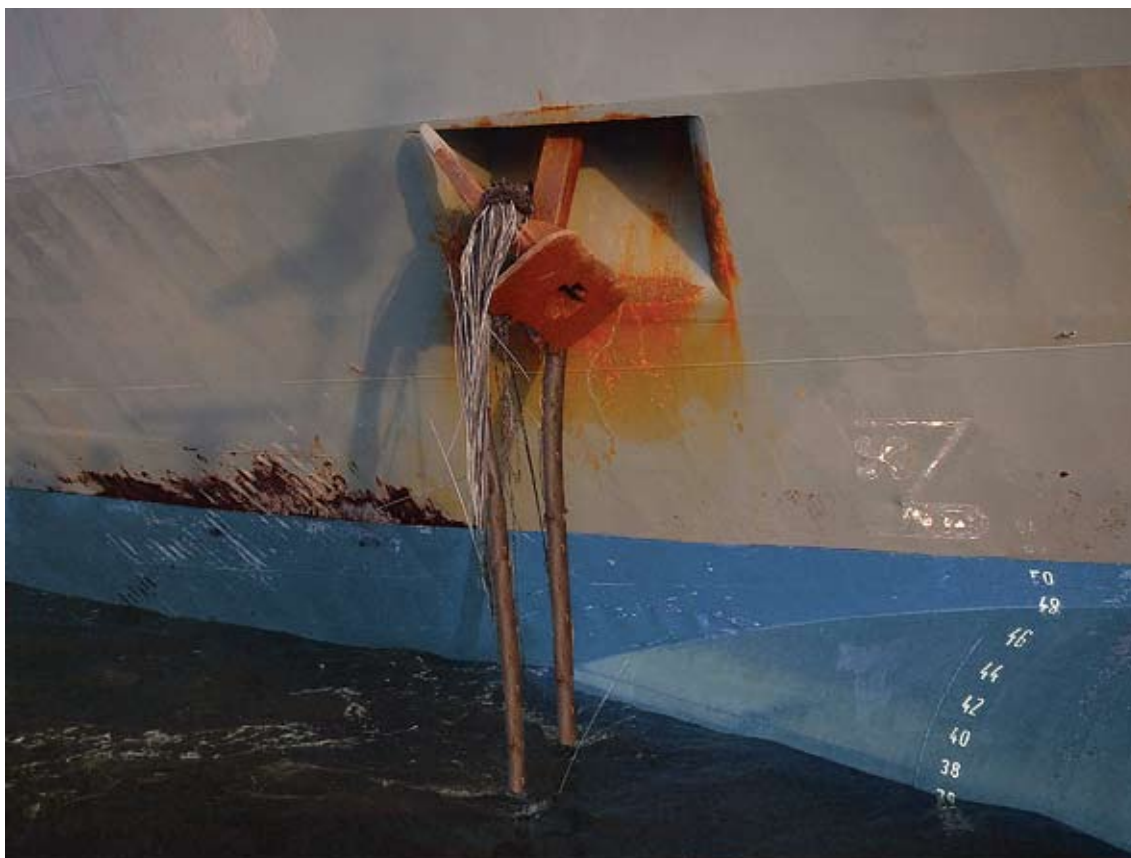
Vessel's anchor, fouled with a power cable
