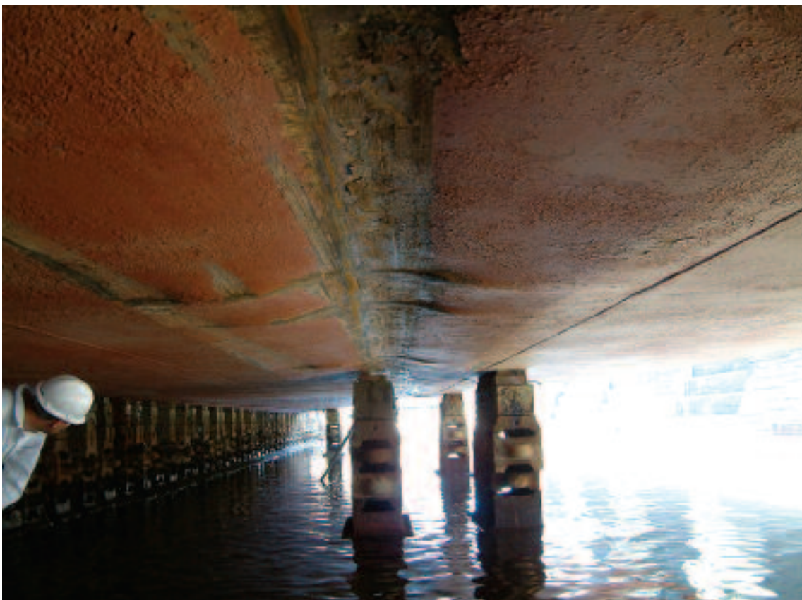
Bottom damage as a result of the grounding
