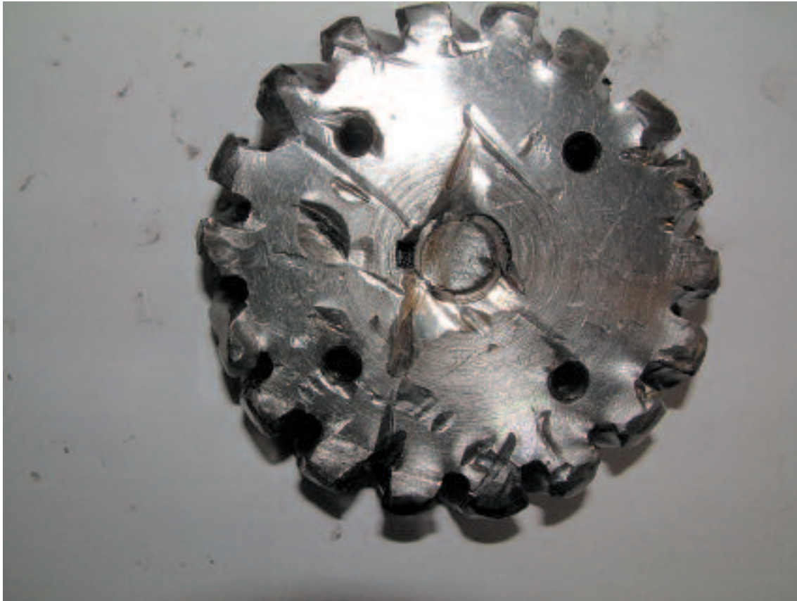
Figure 2 – Sheared drive shaft and pinion
