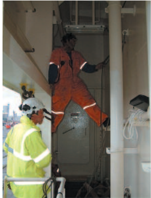
Position of crew for lowering pilot ladder overboard
