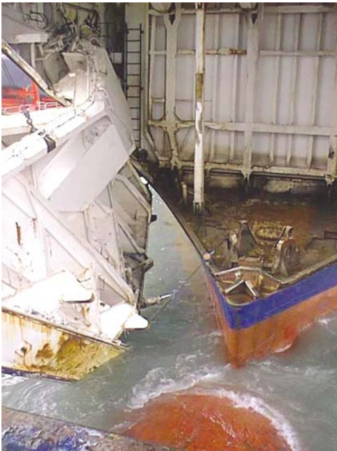
Figure 2: View of damaged starboard bow door
