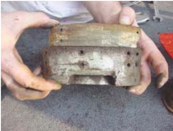
This picture shows the pad and shoe – note the misalignment of the rivet holes
