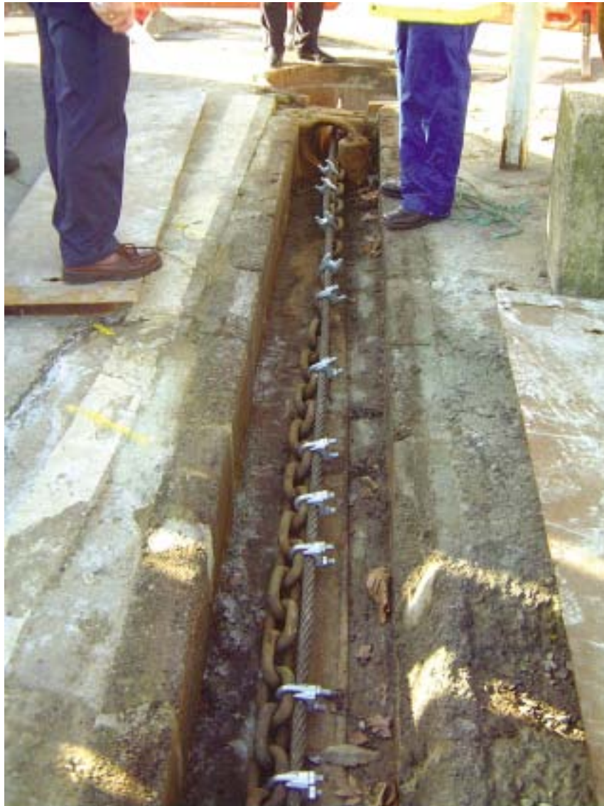
Figure 1 – Before the incident the wire was attached to chain using bulldog clips
