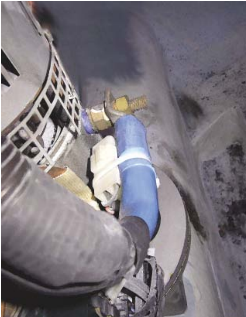
Figure 1: Bow thruster showing exposed power cables and fire damage
