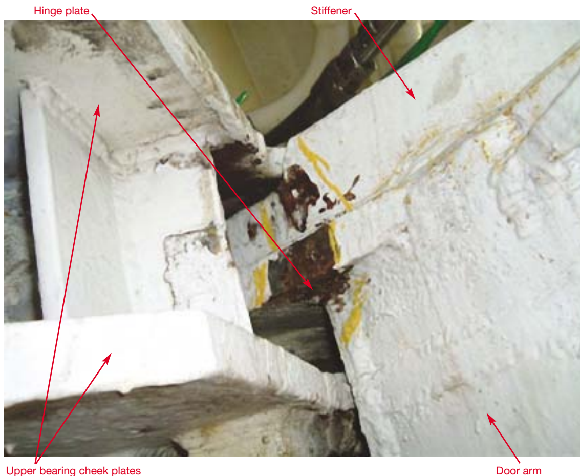
Figure 1a: Starboard door upper bearing arrangement
