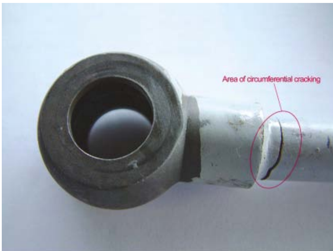
Figure 2: Failed low pressure fuel pipe
