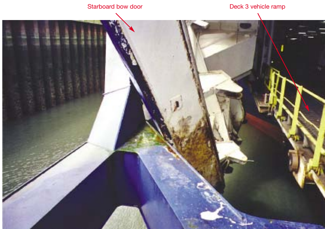
Figure 3b: Starboard door in contact with 'cowcatcher'
