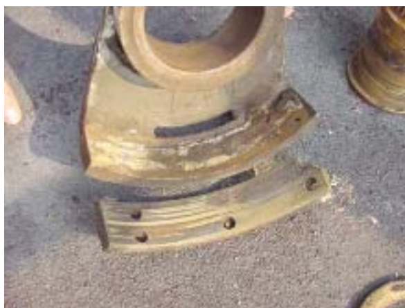
Securing of the pad had been carried out by the use of adhesive over the full face and two rivets at one end
