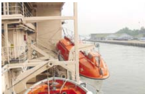
Photograph showing the lifeboat at its position of rest, with the forward gripe trapped and the aft davit arm moved to the lower position. The twisting action wedged the boat as shown
