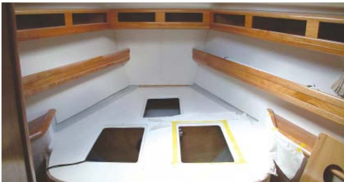
Figure 2: Machinery space with no visible warnings can be easily mistaken for a storage locker
