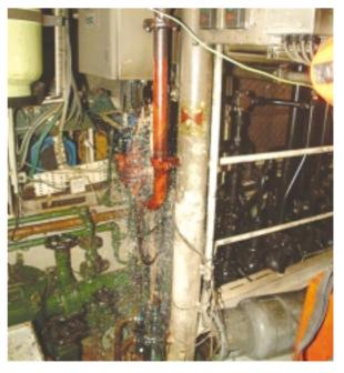
Replicated fuel leakage from main engine duplex fuel filters
