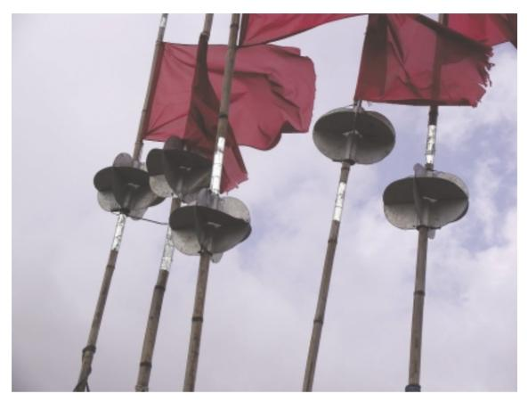
Fishing float radar reflectors
