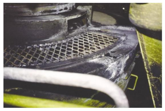
Photograph showing the burnt out clutch
