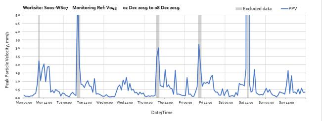
Note: High vibration levels throughout the week were due to local disturbance of the vibration monitor and are not representative of HS2 vibration levels.
