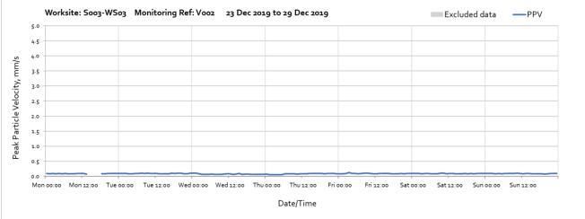
Note: Missing data between 13:00 and 18:00 on Monday 23<sup>rd</sup> December was due to loss of connection from the monitoring station to the data server.
