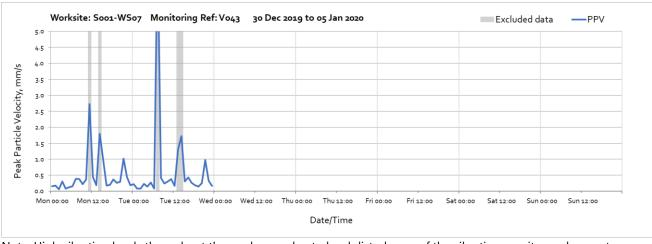
Note: High vibration levels throughout the week were due to local disturbance of the vibration monitor and are not representative of HS2 vibration levels.
