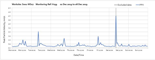
Note: High vibration levels at 08:00 on Saturday 7<sup>th</sup> December were due to local disturbance of the vibration monitor and are not representative of HS2 vibration levels.
