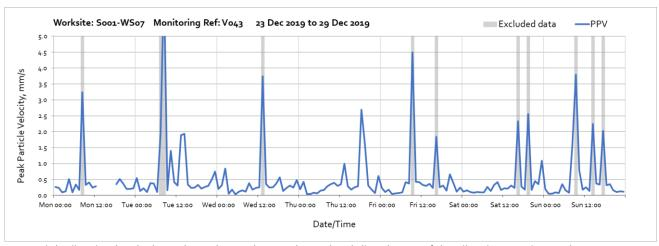
Note: High vibration levels throughout the week were due to local disturbance of the vibration monitor and are not representative of HS2 vibration levels. Missing data between 13:00 and 18:00 on Monday 23<sup>rd</sup> December was due to loss of connection from the monitoring station to the data server.
